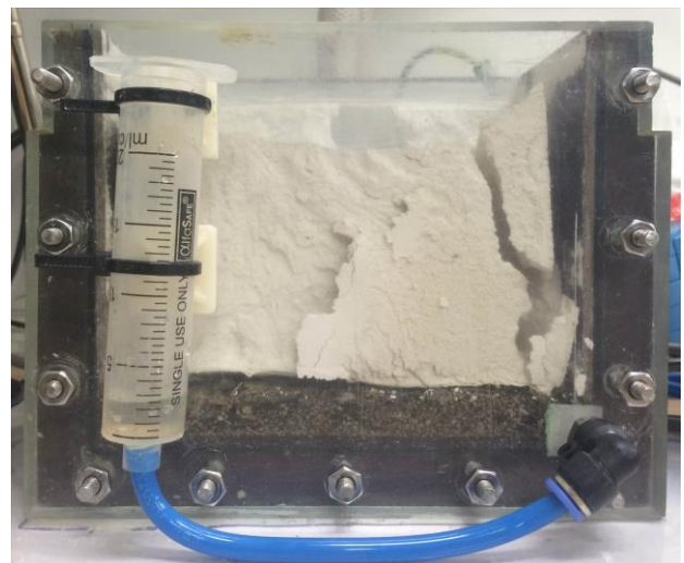
Figure 10. Crack formation. Test T3.
