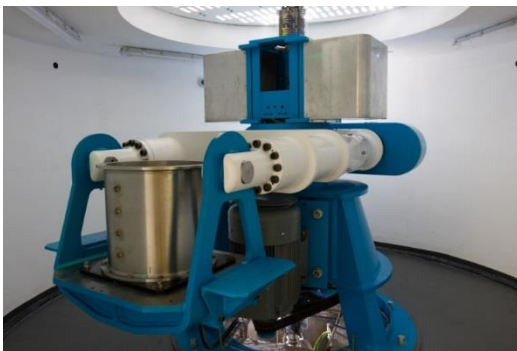
Figure 1. UoS-50gT 4m diameter centrifuge.
