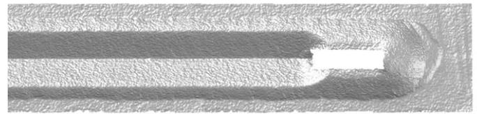
Figure 6. Plan view of typical recombined 3D scan of sand surface in AutoCAD post ploughing.
