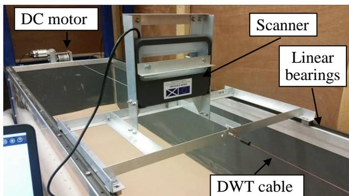
Figure 4. Mounting frame and linear bearings used to allow the scanner to be moved the full length of the model container.
