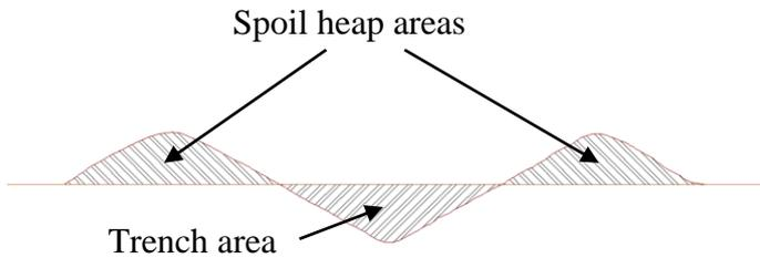
Figure 8. Estimation of the area of each part of the 3D scan surface cross-section using AutoCAD.
