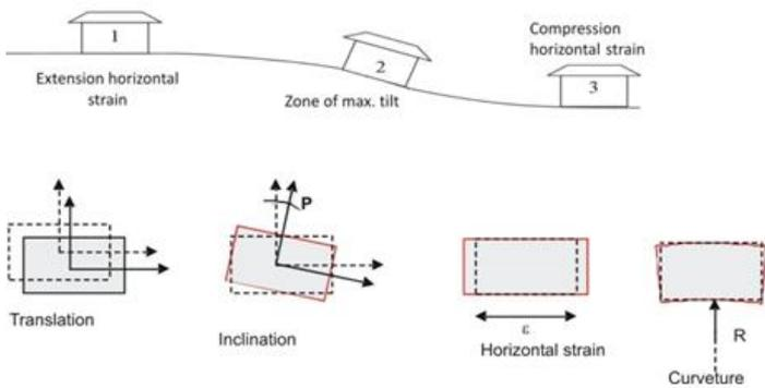
Figure 2. Different types of movement affecting a structure (Deck et al., 2003).
