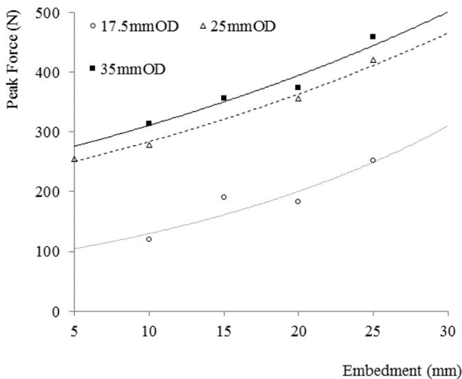
Figure 15. Parallel trend between different casing diameters when the casing embedment is varied in 120mm overburden, data from Tests A, B & C
