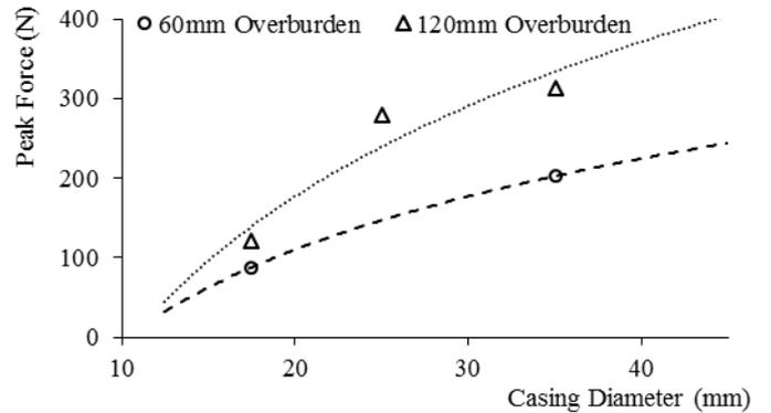
Figure 14. Peak forces when varying overburden heights against casing diameter for constant embedment of 10mm from Tests A & C. Note: A similar trend was observed for constant embedment of 20mm
