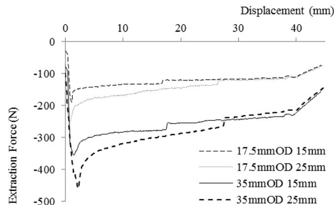
Figure 5: Each casing extraction force in Test B; force decreases as casings are extracted from clay layer at 15mm and 25mm
