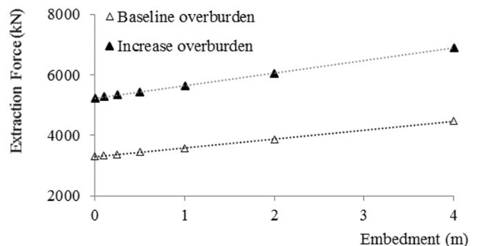
Figure 10: Effects of changes in overburden height on extraction forces
