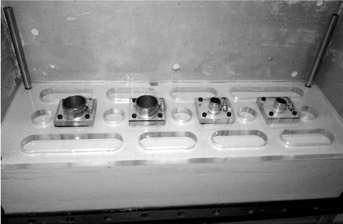
Figure 1: Perspex template placed on clay layer and adjustable steel collars pushed into clay to cut shelf for each required embedment depth (Gorasia et al., 2014)
