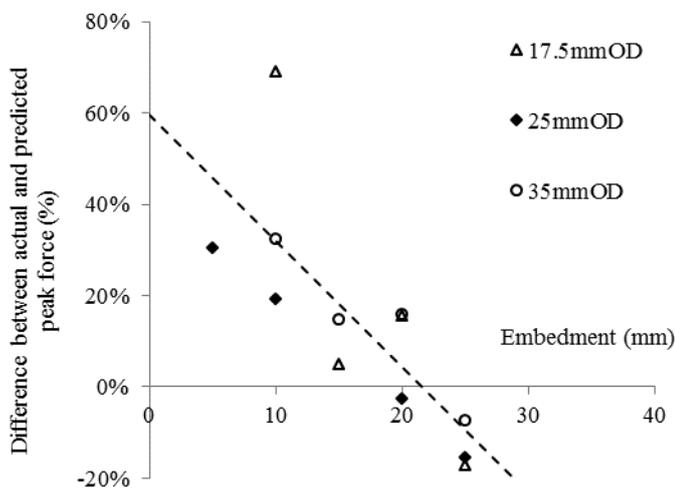
Figure 16. Trend between casing embedment and percentage difference between actual and predicted peak forces
