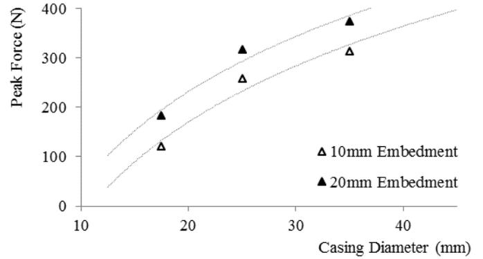
Figure 13: Change in peak force from Tests A & C when doubling embedment from 10mm to 20mm in 120mm overburden. Note: A similar trend was observed for constant overburden of 60mm
