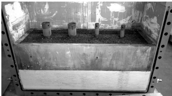
Figure 6: Post-test; casings extracted in Test B
