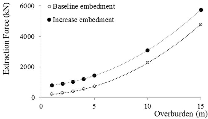
Figure 11: Effect of increasing embedment on extraction forces
