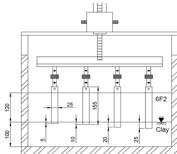
Figure 7: Test C centrifuge model set up
