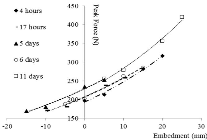
Figure 8: Peak force against embedment depth for varying consolidation periods
