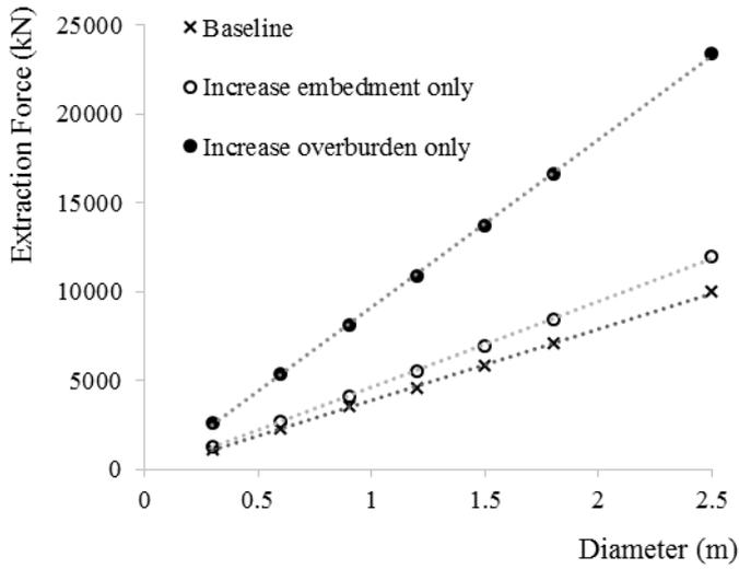
Figure 12: Effects of varying overburden or embedment on casing extraction
