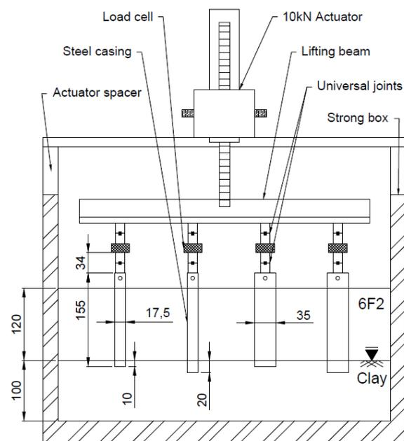
Figure 3: Test A centrifuge set up
