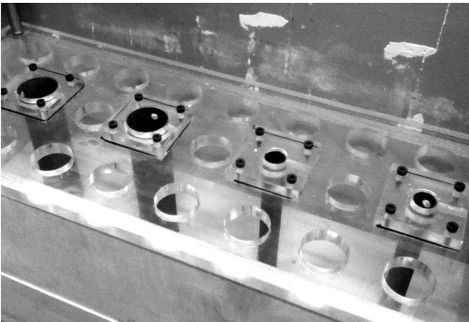
Figure 2: Casings rest on precut sheft and supported at the top by Perspex template hung from top of strongbox prior to placing of 6F2 within plywood former (Gorasia et al., 2014)
