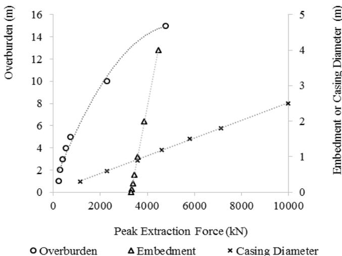
Figure 9: Effect of varying embedment, overburden or casing diameter
