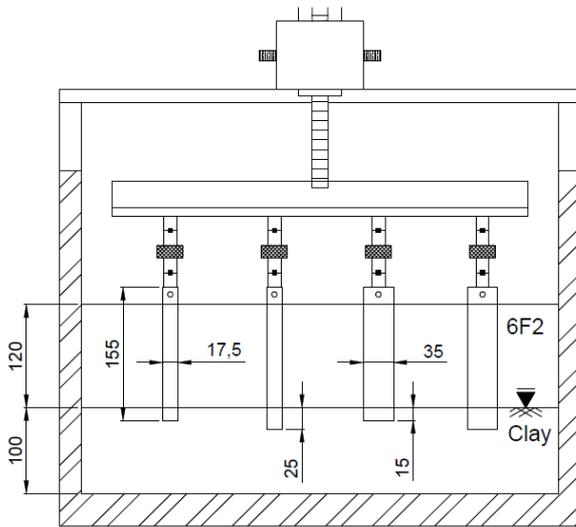
Figure 4. Test B centrifuge set up
