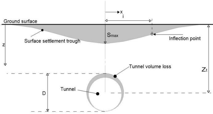
Figure 1. Tunnel volume loss.
