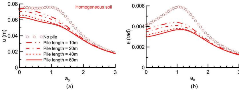
Figure 2. (a) Horizontal displacements and (b) rotation angles of the CCPF in homogeneous soils (from Zhong & Huang 2013).
