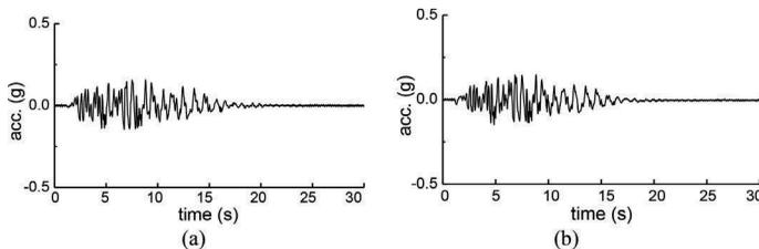
Figure 11. Acceleration time histories of free field at soil surface: (a) test 2; (b) test 3.
