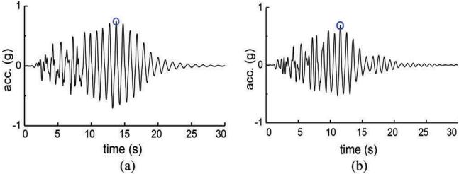
Figure 13. Acceleration time histories of the upper structure: (a) caisson (test 2); (b) CCPF (test 3).
