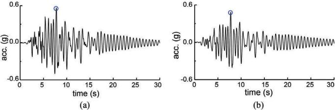
Figure 14. Acceleration time histories of the foundation: (a) caisson (test 2); (b) CCPF (test 3).
