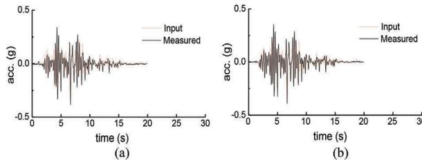
Figure 10. Acceleration time histories of free field soil at ground base: (a) test 2; (b) test 3.
