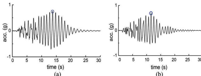
Figure 12. Acceleration time histories of upper structure on single pile: (a) test 2; (b) test 3.
