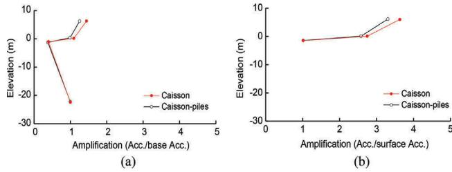
Figure 15. Amplifying of acceleration in soil layer, foundation and upper structure: based on (a) base acceleration and (b) surface acceleration.
