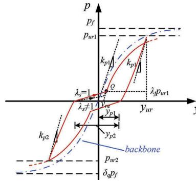
Figure 17. Schematic of unloading and reloading curves (from Huang et al. 2018).
