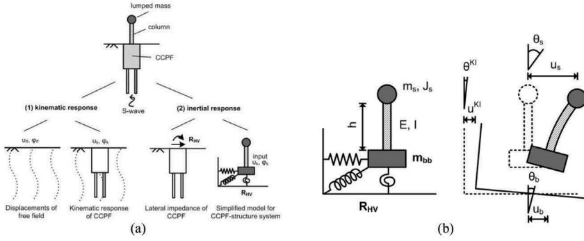
Figure 3. (a) Illustration of the kinematic response and inertial response and (b) a simplified analytical model of a CCPF-structure system(from Zhong & Huang 2014).
