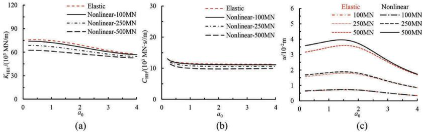
Figure 5. Dynamic responses of CCPF: (a) stiffness; (b) damping; (c) horizontal displacement.
