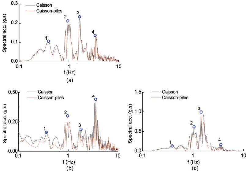
Figure 16. Fourier amplitude spectra of acceleration-time histories: (a) soil surface; (b) foundation; (c) upper structure.
