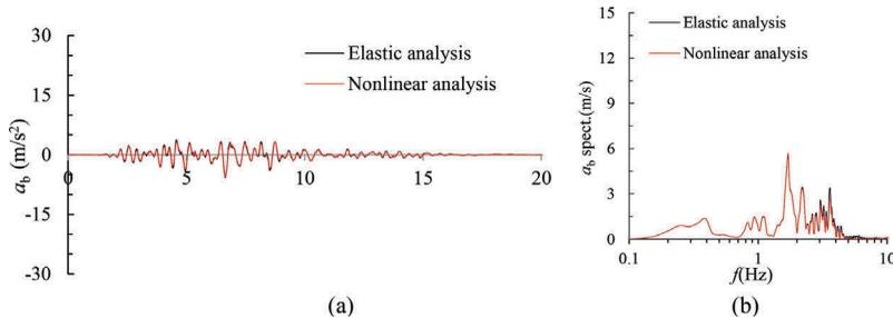
Figure 7. (a) Acceleration time histories and (b) acceleration amplitude spectrum at the foundation.
