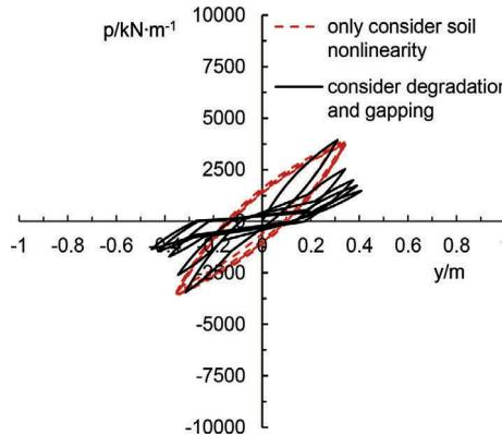
Figure 18. Comparison of the horizontal soil reaction-displacement loops at the selected depth  $z=10\text{m}$  (from Huang et al. 2018).
