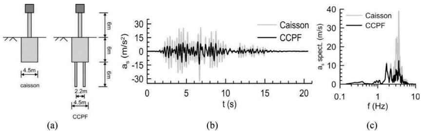
Figure 4. (a) CCPF-structure model; (b) time history of the acceleration of the superstructure; (c) acceleration spectrum of the super structure (from Zhong & Huang 2014).
