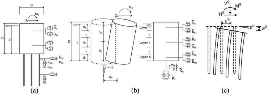
Figure 1. Winkler models for lateral responses of (a) CCPF; (b) caisson; (c) pile groups with rigid cap (from Zhong & Huang 2013).
