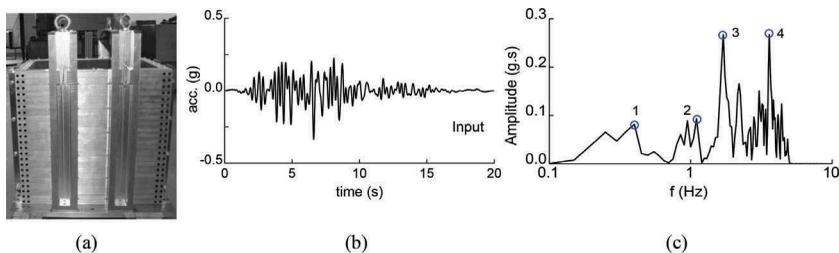
Figure 8. (a) Laminar box; (b) the input acceleration time history; (c) the acceleration response spectra.
