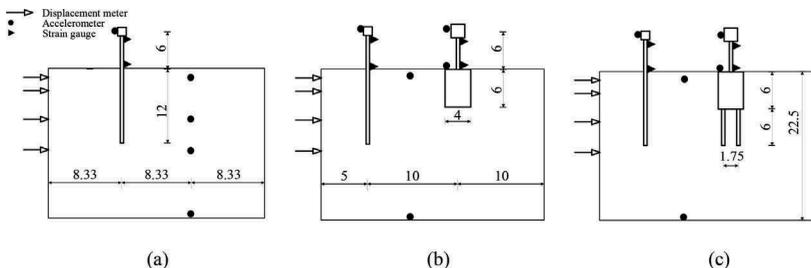
Figure 9. Schematic of test layouts (a) test 1; (b) test 2 - caisson; (c) test 3 - CCPF.
