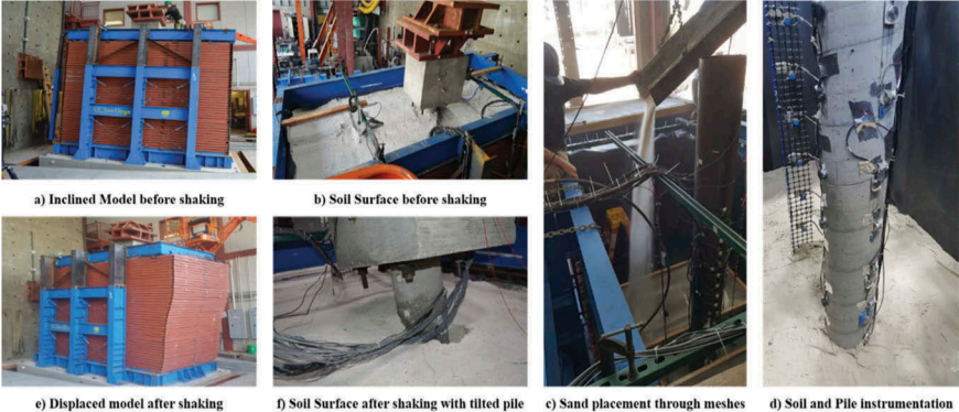
Figure 3. Construction process for test 5 (2.90 m high)
