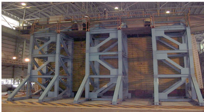
Figure 4. NIED Japan mildly inclined large laminar container on shake table
