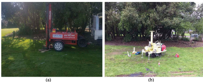
Figure 9. Field testing conducted in Whakatane (WHA-1 site): (a) CPT and sCPT; and (b) SDS test.
