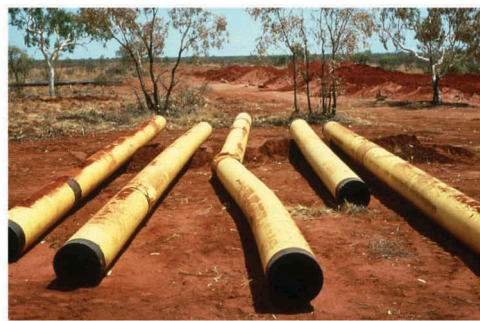
Figure 1. Failure of an API.5L X60 steel gas pipe during the 1999 Tennant Creek, Australia earthquake (source: Geosciences Australia).
