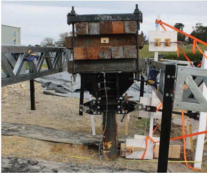
Figure 2. Pile shaft with head mass, instrumentation, and lateral load attachment point.
