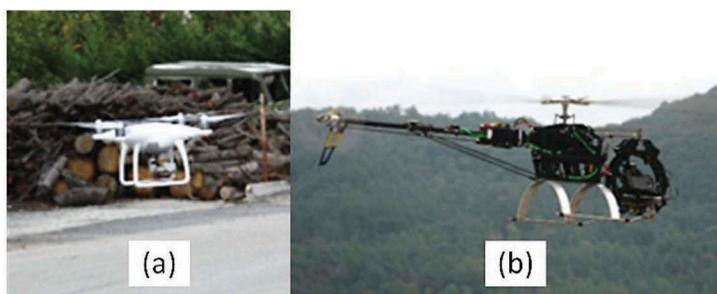
Figure 3. UAVs used for imaging of landslides during 2016 Central Italy reconnaissance
