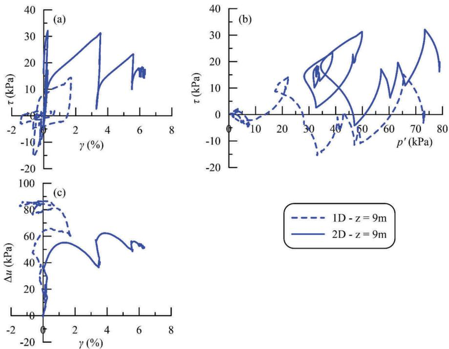
Figure 8. Stress strain curves (a), stress paths (b) and excess pore pressures (c) for 1D and 2D analyses.
