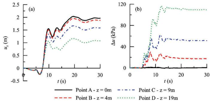
Figure 6. Horizontal displacements (a) and excess pore water pressure (b) for different depths.
