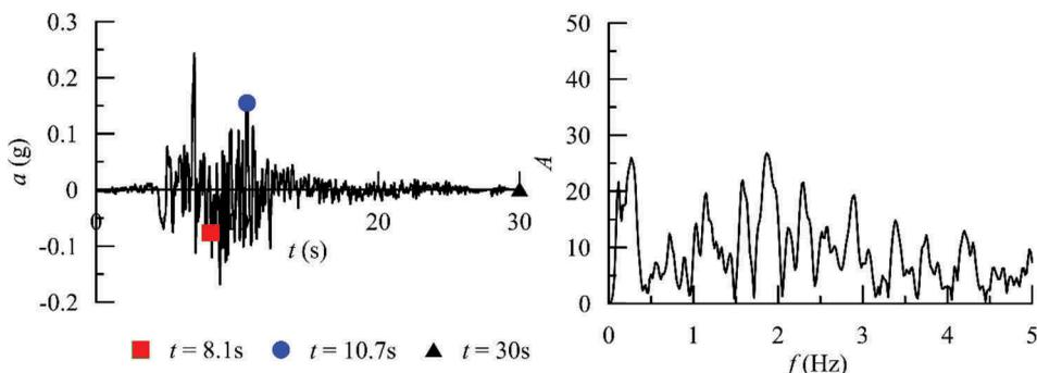
Figure 2. Acceleration time history and Fourier spectrum of the Kocaeli (1999) earthquake.
