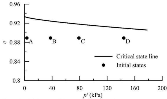
Figure 3. Initial states of the sand at different depths.
