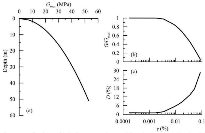
Figure 4. Profile of  $G_{max}$  with depth (a), secant shear modulus reduction curves (b) and variation of damping with shear strains (c).
