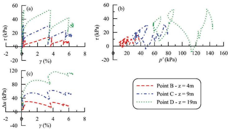
Figure 7. Stress strain curves (a), stress paths (b) and excess pore water pressure (c) for different depths.
