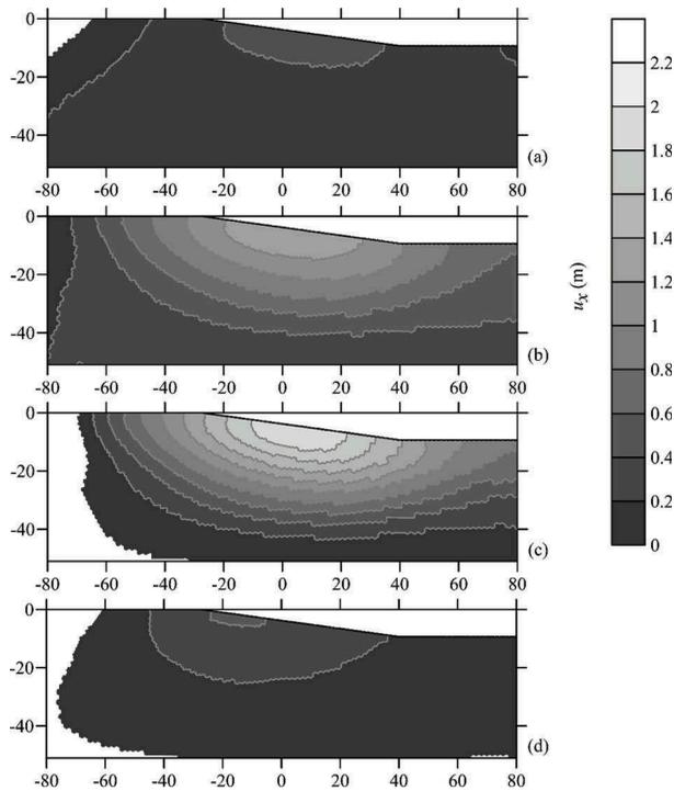
Figure 5. Horizontal displacements contour map at  $t = 8.1$ s (a),  $t = 10.7$ s (b),  $t = 30$ s (c) and at  $t = 30$ s for the drained analysis (d).
