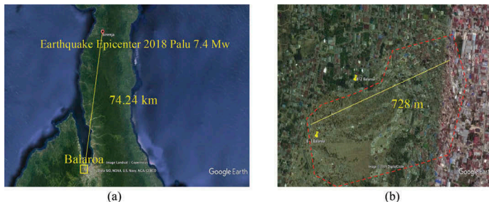
Figure 4. The location (a) and the dimension of lateral ground movement of Balaroa (Google Earth, 2019).
