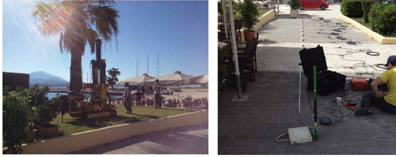
Figure 6. (a) DPT performed in a planter box at the Lixouri Port and (b) MASW performed next to the planter box.
