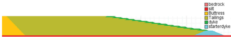
Figure 3. Model of the tailings impoundment used for the numerical simulations, L = 497 m and H = 44 m; the starter dike is 10 m high.
