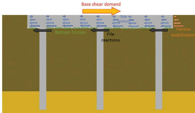
Figure 3. Mechanisms contributing to the lateral stability of a pile foundation system.
