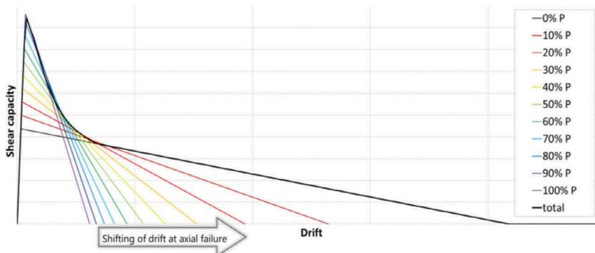
Figure 4. Interaction diagram indicating the effect of decreasing axial load on shear failure behaviour.
