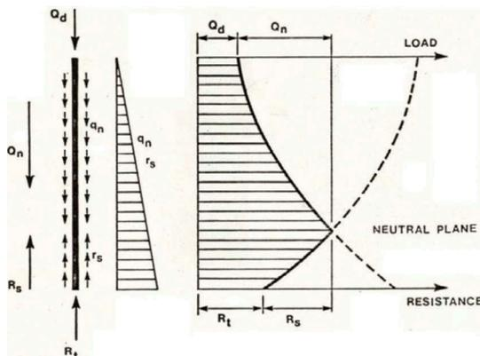
Figure 1. Pile equilibrium state comprising both tip and shaft resistance.
