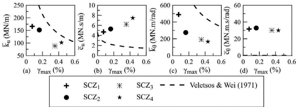
Figure 4. Effect of maximum shear strain of the soil during different seismic events on the average impedance functions and the theoretical impedance functions, developed by Veletsos & Wei (1971): (a) lateral stiffness; (b) lateral dashpot coefficient; (c) rocking stiffness; (d) rocking dashpot coefficient.
