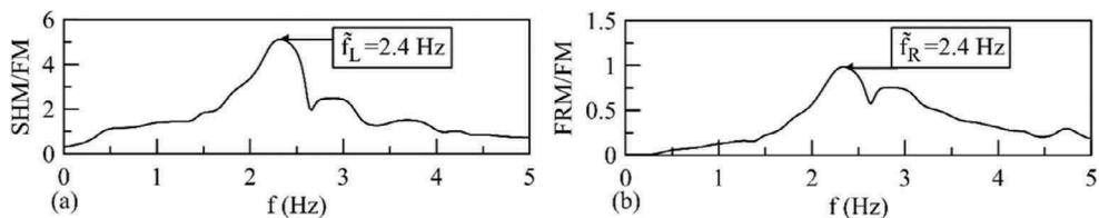
Figure 2. The transfer function of the physical model, when excited by the SCZ<sub>1</sub>: (a) structure transfer function; (b) foundation rocking transfer function.
