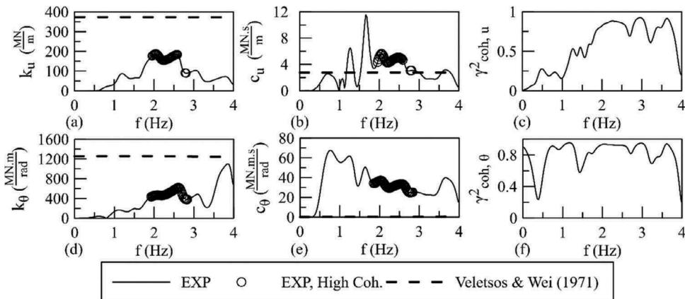
Figure 3. Comparison of the experimental impedance function of the physical model with the theoretical impedance function developed by Veletsos & Wei (1971), when it was excited with SCZ<sub>1</sub> motion: (a) lateral stiffness; (b) lateral dashpot coefficient; (c) coherence of lateral impedance function; (d) rocking stiffness; (e) rocking dashpot coefficient; (f) coherence of rocking impedance function.
