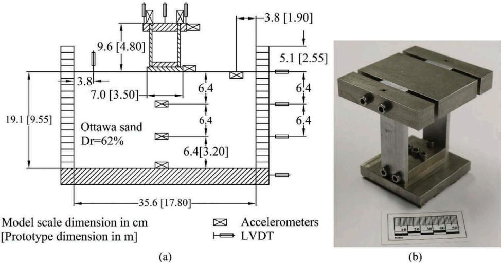
Figure 1. (a) Schematic and instrumentation layout of the centrifuge experiment; (b) photograph of the structure physical model.
