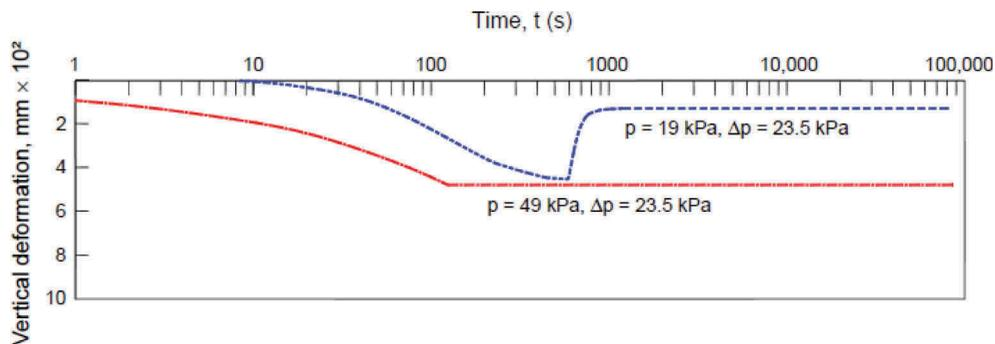
Figure 8. Comparison between two soil samples with different consolidation stress.
