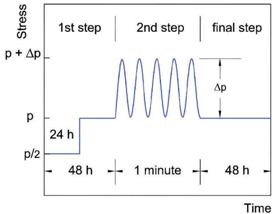
Figure 4. Testing loading sequence.
