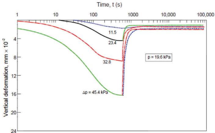
Figure 7. Vertical deformation induced in one-dimensional cyclic loading.
