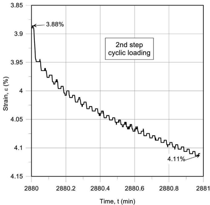
Figure 6. Time-strain curve under cyclic loading.
