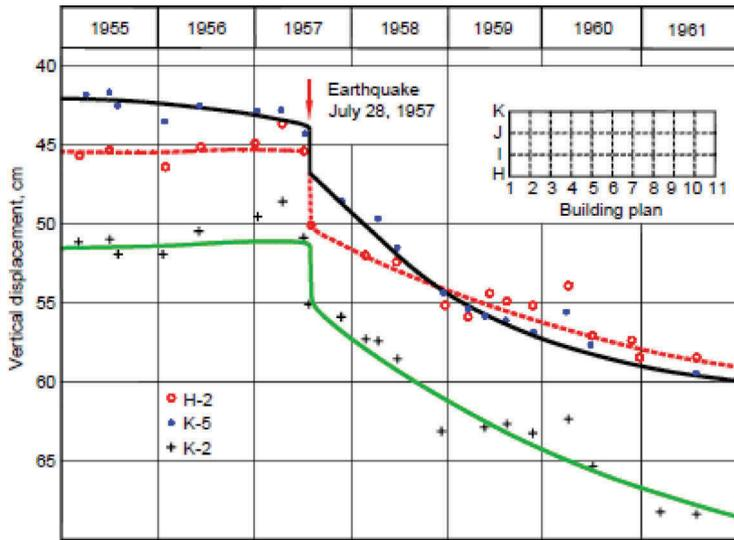
Figure 1. Effect of July 28, 1957 Guerrero earthquake on the settlement of a building (Zeevaert 1973).
