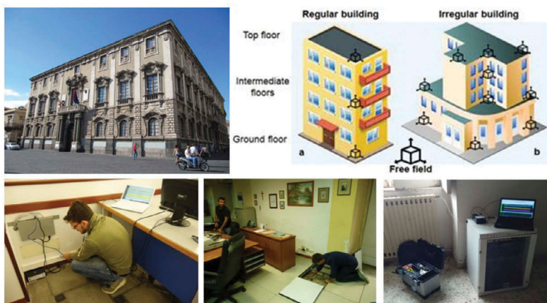
Figure 4. Operation of installation and configuration of a monitoring station at the ground floor of the 18th century “Elefanti Palace” located in the main square of Catania. Schemes for the sensors’ distribution into edifices: a) minimum necessary requirements for a regular multi-storey building, and b) ideal extensive installations for an irregular masonry building.
