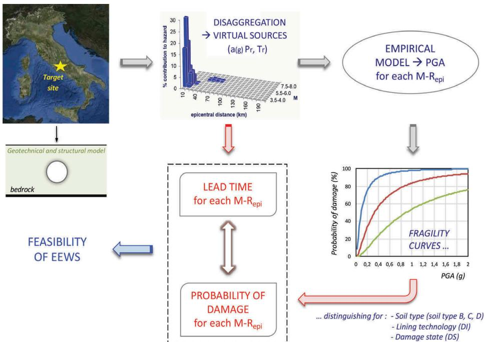
Figure 2. Layout of the proposed method based on the disaggregation of the PSHA to evaluate the probability of seismic damage of underground tunnels and the related feasibility of seismic EWS. (Modified after Fabozzi et al. 2018).
