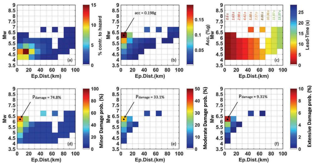
Figure 4. (a) Disaggregation (INGV, <http://zonesismiche.mi.ingv.it>), (b) acceleration and (c) lead-time maps of target site of Bologna HS railway passage and maps of probability of damage for (d) minor, (e) moderate and (f) extensive damage level ( $P_r = 63\%$ ). (Modified after Fabozzi et al. 2018).
