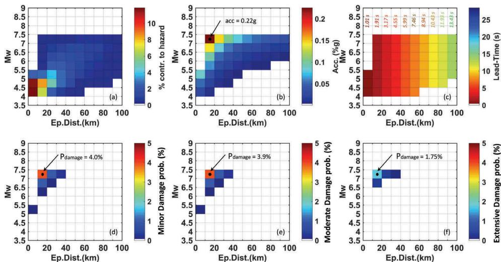
Figure 5. (a) Disaggregation (INGV, <http://zonesismiche.mi.ingv.it>), (b) acceleration and (c) lead-time maps of target site of La Botte HS railway tunnel and maps of probability of damage for (d) minor, (e) moderate and (f) extensive damage level ( $P_r = 63\%$ ). (Modified after Fabozzi et al. 2018).
