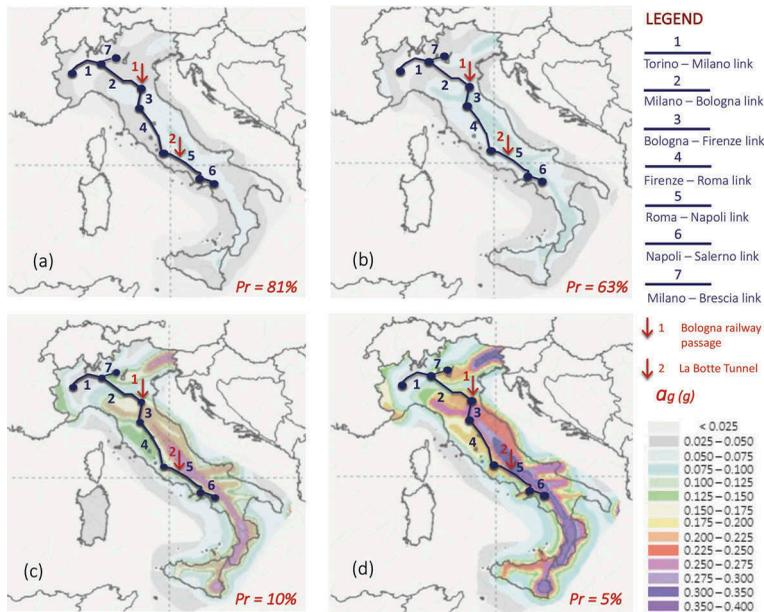
Figure 3. Italian high speed rail system (operational) combined with the hazard maps for a probability of exceedance equal to (a) 81% (return period TR = 30 y), (b) 63% (return period TR = 50 y), (c) 10% (return period TR = 475 y), and (d) 5% (return period TR = 975 y). (Hazard maps extracted from INGV, <http://zonesismiche.mi.ingv.it>). (Modified after Fabozzi et al. 2018).
