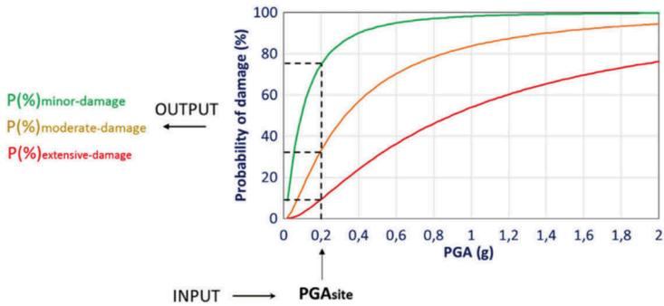
Figure 1. Schematic application of the fragility curves. (Modified after Fabozzi et al. 2018).
