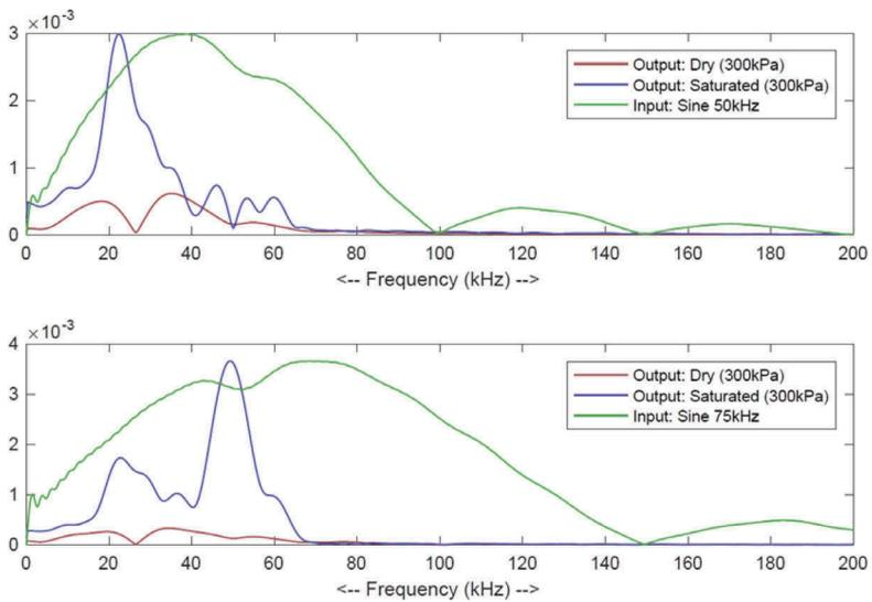
Figure 6. Frequency spectra for BE signals for 50kHz and 75kHz input frequencies, for dry and saturated conditions, at 300 kPa confining stress
