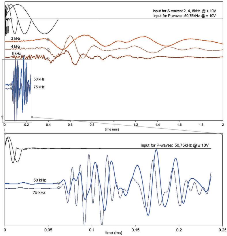
Figure 5. BE measurements for S- and P-waves: saturated conditions, at 300 kPa isotropic confinement
