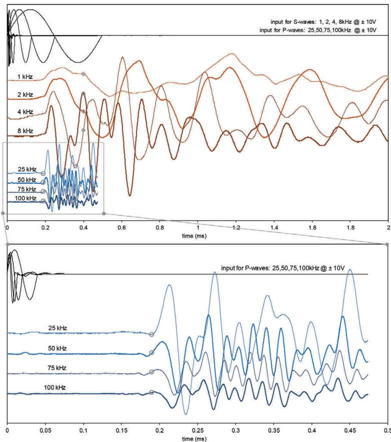
Figure 4. BE measurements for S- and P-waves: dry conditions, at 300 kPa isotropic confinement
