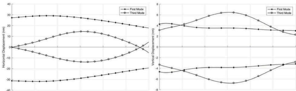
Figure 2. First and third vibration modes for horizontal and vertical displacements on top of the BE, along its width.
