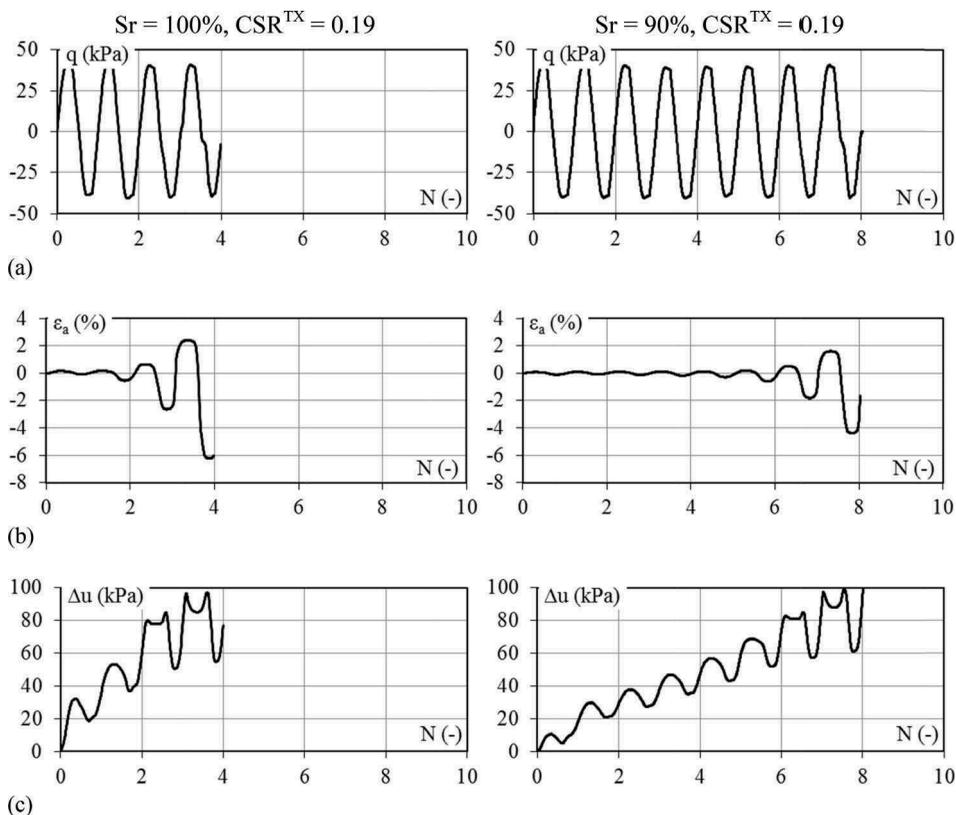
Figure 3. Undrained CTX tests on saturated (left side) and unsaturated ( $Sr = 90\%$ , right side) samples: (a) stress deviator  $q$ , (b) axial strain  $\epsilon_a$  and (c) excess pore pressure  $\Delta u$  as a function of number of cycles  $N$ .
