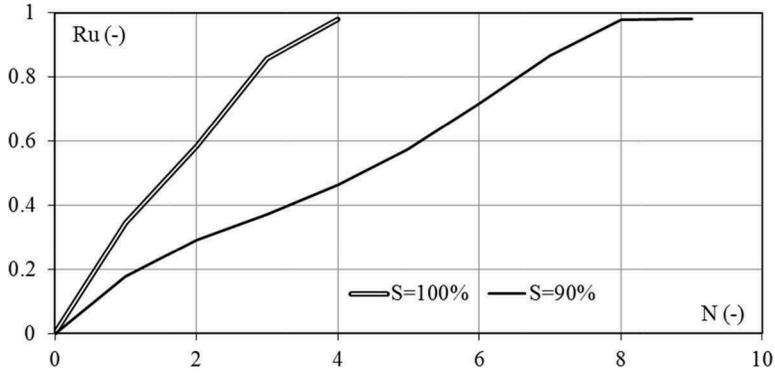
Figure 4. Pore pressure ratio measured during two undrained CTX tests carried out applying the same cyclic stress ratio ( $CSR_{TX} = 0.19$ ) on a saturated and a partially saturated sample.
