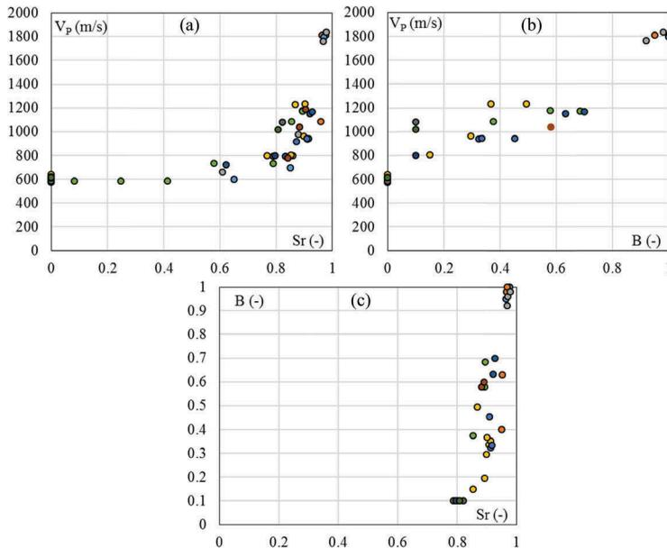
Figure 2. (a) Compression wave velocity V<sub>P</sub> vs. the degree of saturation Sr, (b) V<sub>P</sub> vs. Skempton parameter B; (c) B vs. Sr.
