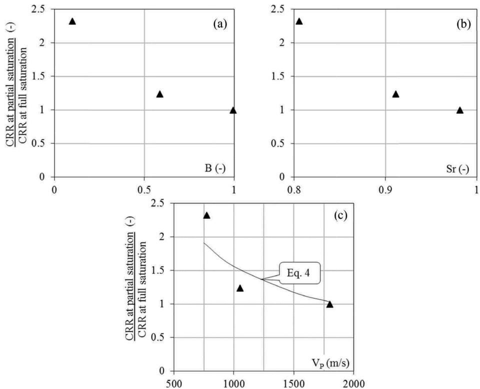
Figure 5. Cyclic resistance CRR of unsaturated samples normalized to the cyclic resistance of fully saturated samples plotted vs. (a) the Skempton B parameter, (b) the degree of saturation  $Sr$ , and (c) the compression wave velocity  $V_p$ .
