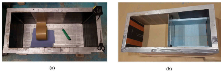
Figure 4. Model preparation: (a) method used to reduce sidewall friction; (b) installed facing using temporary supports
