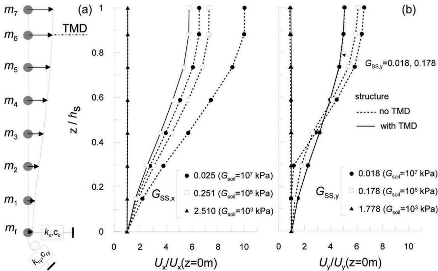
Figure 3. Profiles of the horizontal displacements of the structure in the X and Y directions, figures (a) and (b) respectively, obtained in correspondence of the relative fundamental periods.
