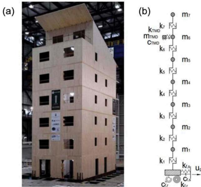
Figure 1. (a) View of the seven-storey building tested in the SOFIE project and (b) schematic representation of the simplified 3D numerical model accounting for soil-structure interaction.
