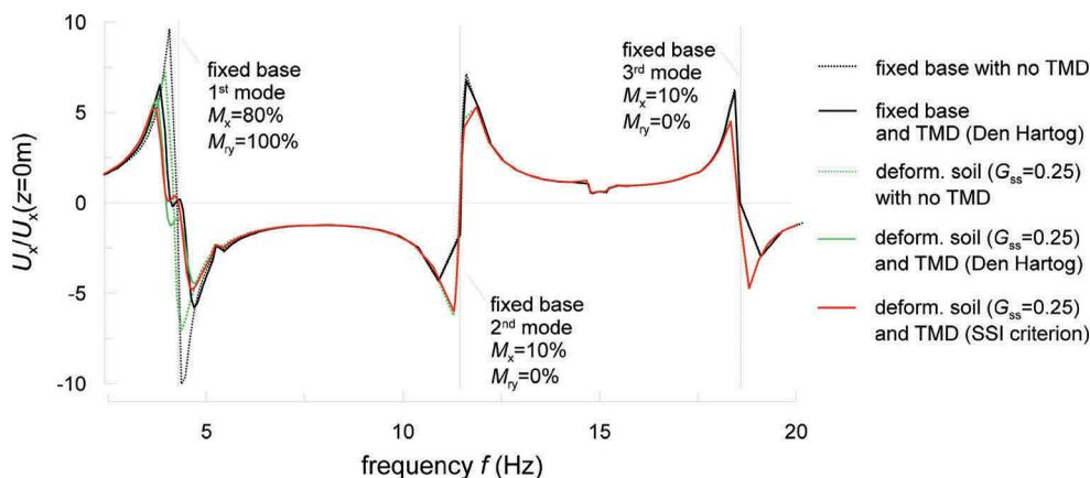
Figure 7. Amplification of the normalised displacement of the mass  $m_6$  in the X direction plotted as a function of the frequency  $f$ : comparison between the Den Hartog and the SSI design criteria of the TMD.
