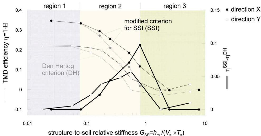
Figure 6. TMD designed considering the fundamental period of the soil-structure system: TMD efficiency  $\eta$  plotted as a function of the relative stiffness  $G_{SS}$  for the X and Y directions.
