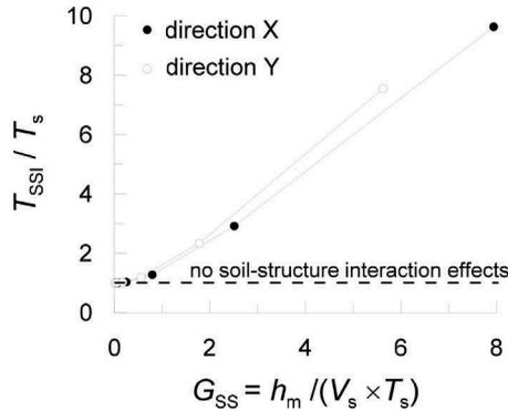
Figure 2. Period elongation plotted as a function of the structure-to-soil relative stiffness  $G_{\text{SS}}$ .
