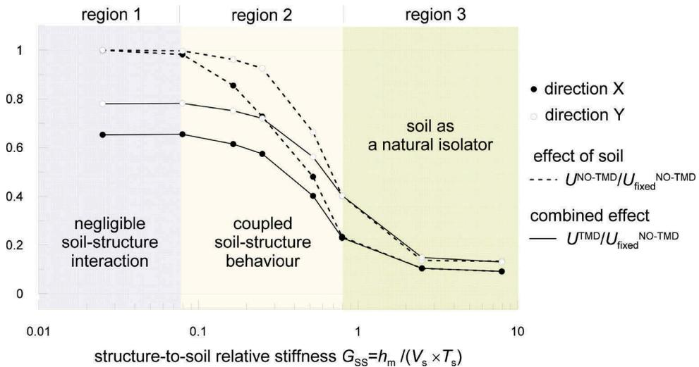
Figure 5. Effect of the soil deformability and of the TMD, the latter designed according to the Den Hartog's criterion, on the maximum displacement of the structure as a function of the structure-to-soil relative stiffness  $G_{SS}$ , in the X and Y directions.
