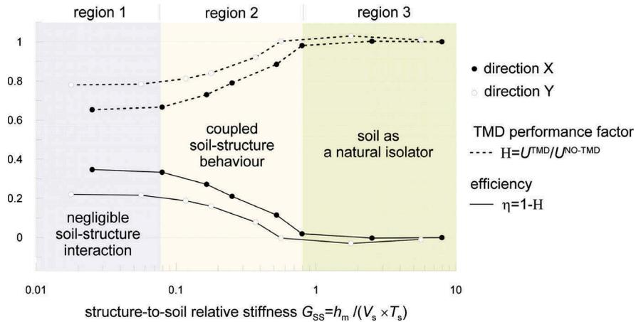
Figure 4. TMD designed according to Den Hartog's criterion: TMD performance factor  $H$  and efficiency parameter  $\eta$  plotted as a function of the relative stiffness  $G_{SS}$  for the X and Y directions.
