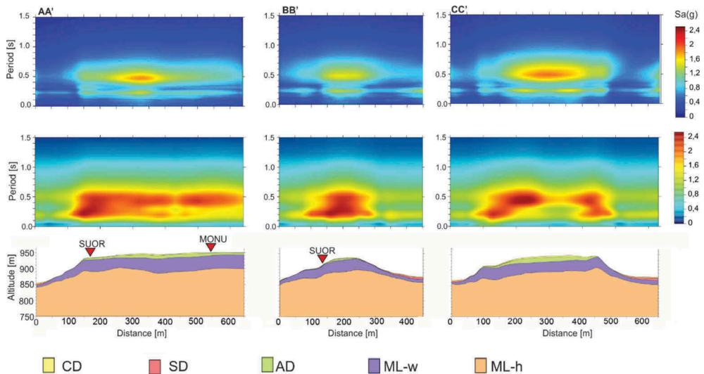
Figure 7. Results from 2D-FEM (top) and hybrid analysis (middle) on the analysed cross-sections (bottom) in terms of spectral acceleration  $S_a$  vs period along the three analyzed cross-sections.
