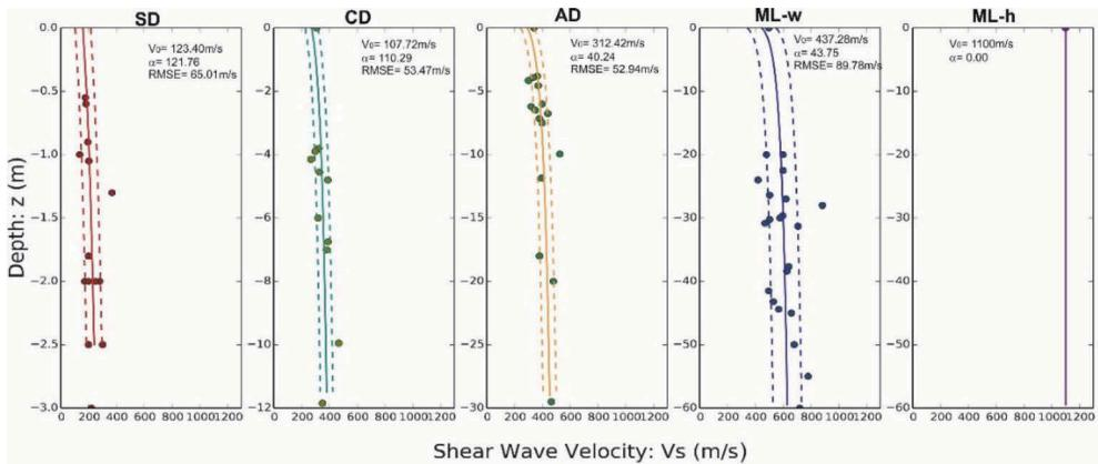
Figure 5.  $V_s$ - $z$  profiles obtained in pre-processing field data by module 1 of SiSeRHMap.
