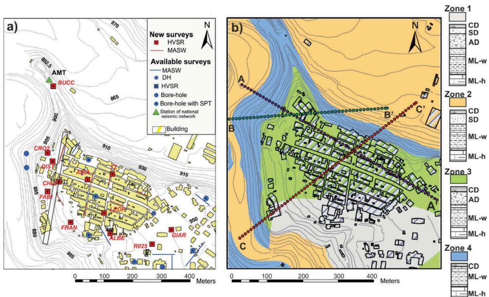
Figure 1. Surveys map and HVSR station sites (a); geo-lithological zonation map obtained by using GIS modeling in SiSeRHMap and cross-sections used in the 2D-FEM analysis (b).
