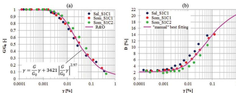
Figure 4. Resonant Column experimental data from CD lithological Unit samples and best fitting  $G/G_0$ - $\gamma$  (a) and  $D$ - $\gamma$  (b) curves.
