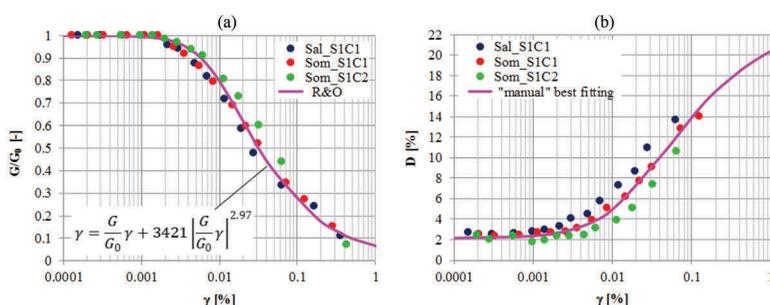
Figure 3. Normalized shear modulus (left) and damping ratio (right) curves.
