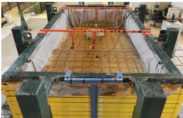
Figure 2. Top view of physical model in laminar box on shake table before shaking
