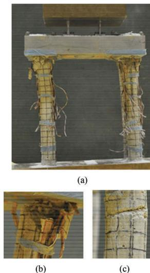
Figure 7. Pile member damage.
