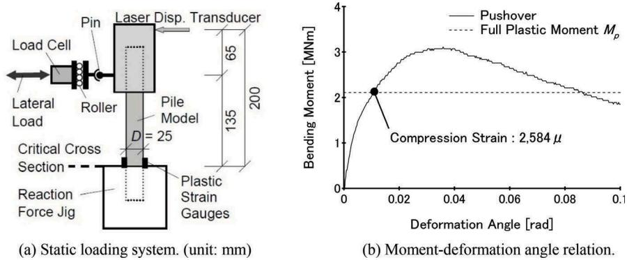
Figure 2. Static loading test of the pile model.
