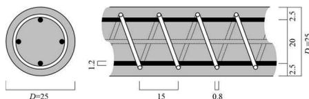
Figure 1. Cross section of the pile model. (unit: mm)
