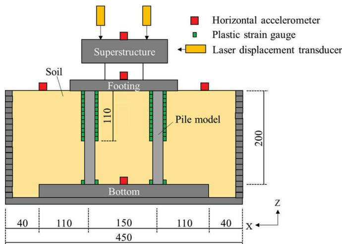
Figure 3. Experimental model for the centrifuge shaking table test. (unit: mm)
