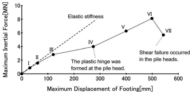
Figure 8. Maximum inertial force at each shaking.
