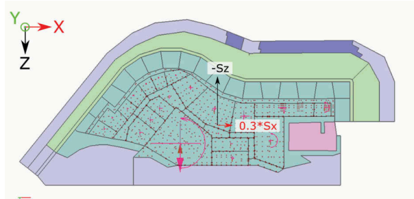
Figure 6. Kinematic load case for the 3D model and illustration of the efforts from the superstructures (inertial loading).
