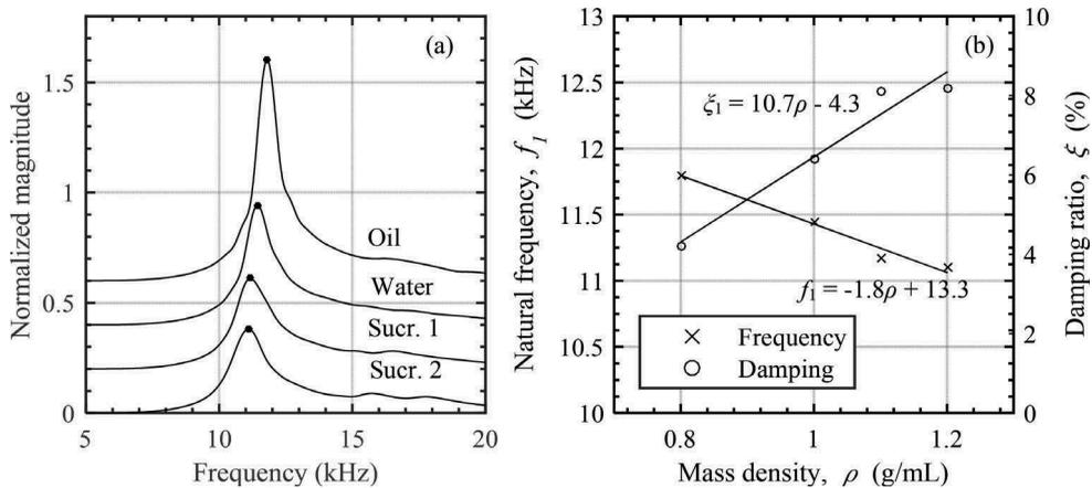
Figure 4. (a) Frequency spectra of the  $T_x$  responses in liquids (b)  $f_1$  and  $\xi_1$  of the  $T_x$  against  $\rho$  of the liquids.
