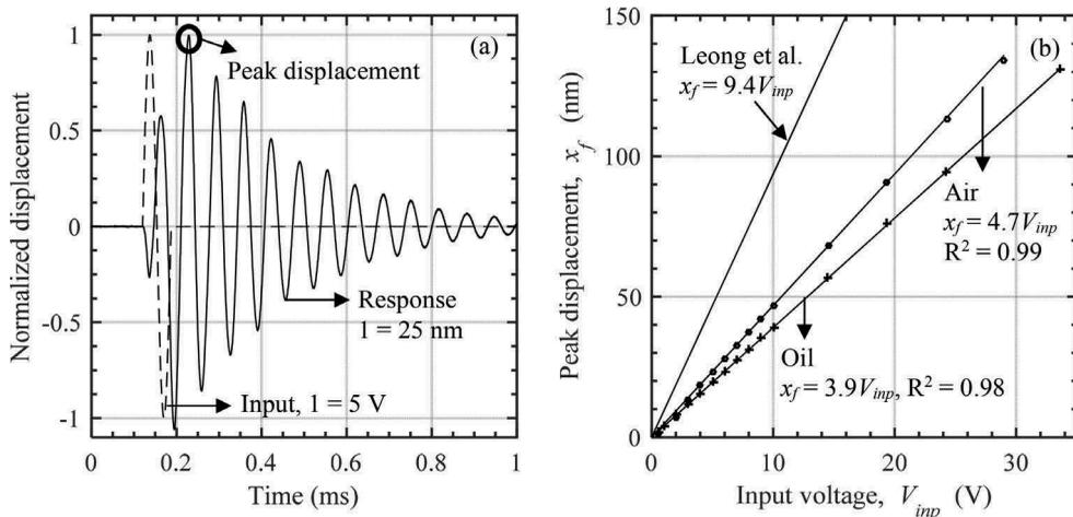
Figure 3. (a) A typical  $T_x$  response in air to a sine pulse; (b) peak  $T_x$  response displacement vs input voltage.
