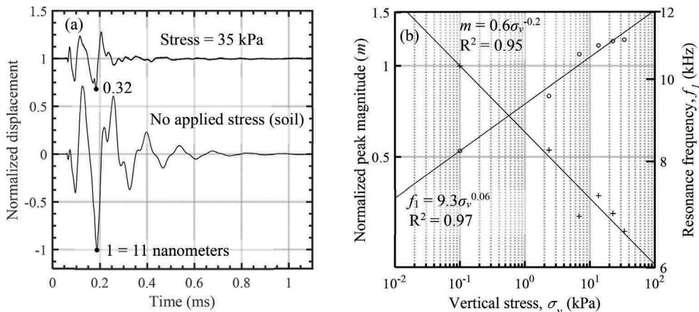
Figure 5. (a)  $T_x$  responses in transparent soil with and without stress; (b)  $m$  and  $f_1$  vs  $\sigma_v$  in the soil
