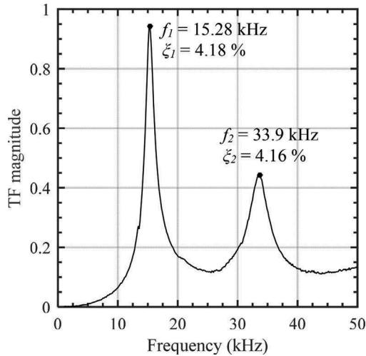
Figure 2. Transfer function of the transmitter ( $T_x$ ) in air computed from  $T_x$  response to a sinusoidal sweep.
