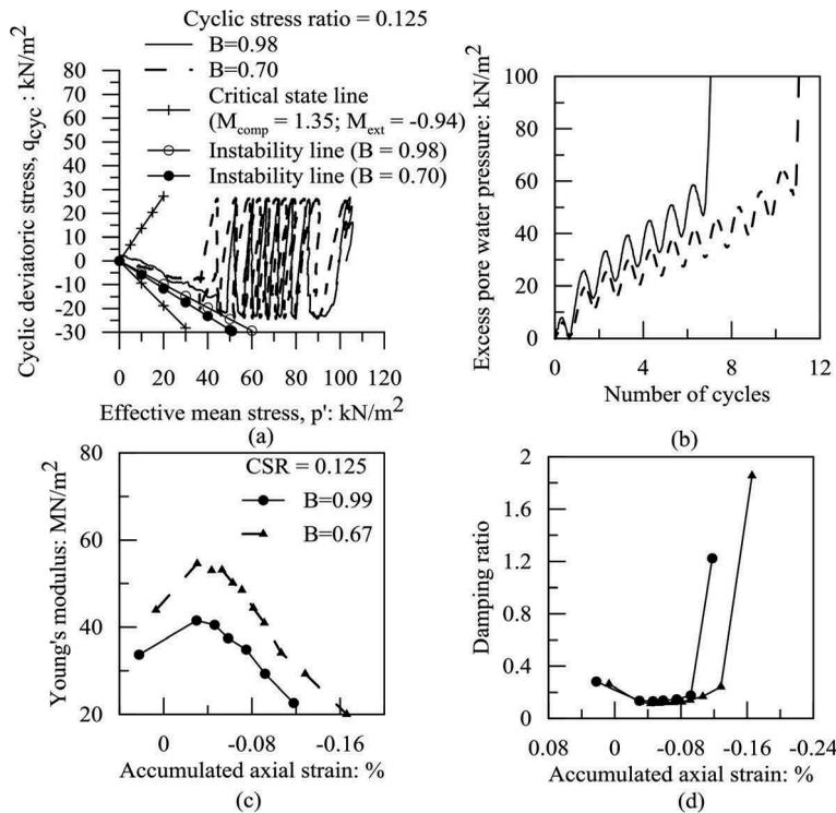
Figure 8. Effect of desaturation on: (a) cyclic stress path; (b) generation of excess pore pressure; (c) stiffness degradation; (d) accumulation of axial strain against damping ratio.
