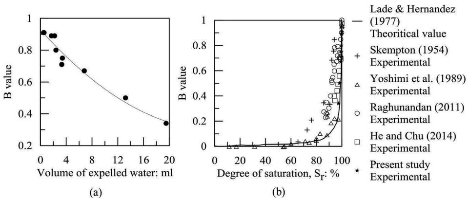
Figure 2. (a) Change in pore pressure coefficient B with expel of water during desaturation; (b) relationship between B and degree of saturation.
