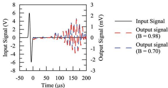
Figure 3. Comparison between saturated and desaturated sand sample using bender element test.
