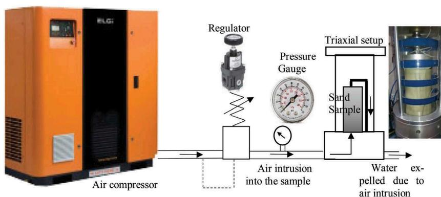
Figure 1. Desaturation procedure used in triaxial tests.
