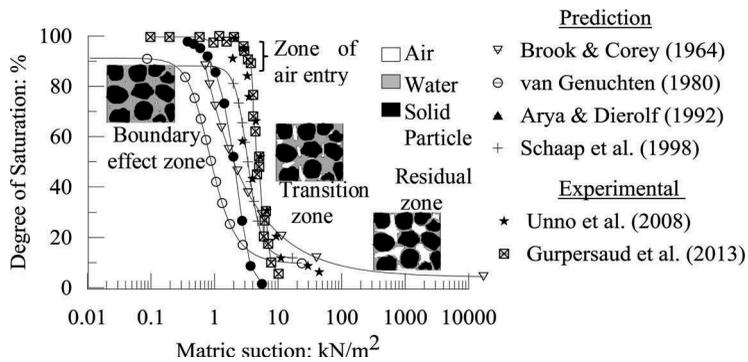
Figure 4. Soil water characteristic curve (SWCC) for Gujarat sand.
