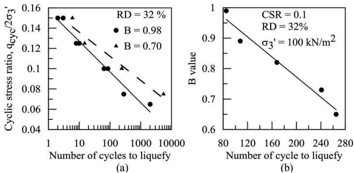
Figure 7. (a) Effect of desaturation on the cyclic strength of Gujarat sand; (b) B value vs number of cycles to reach liquefaction.
