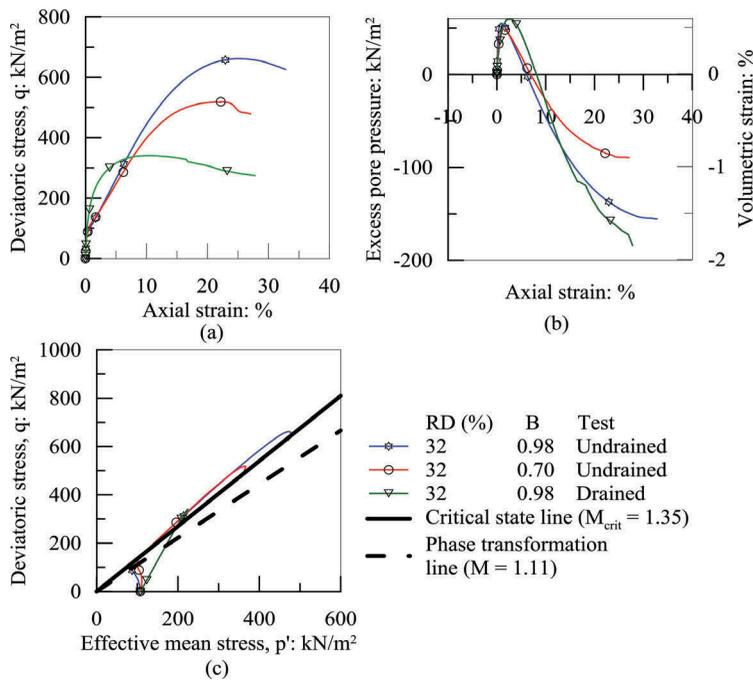
Figure 6. Effect of desaturation on: (a) stress strain behaviour; (b) excess pore pressure variation; (c) stress path in monotonic triaxial extension test.
