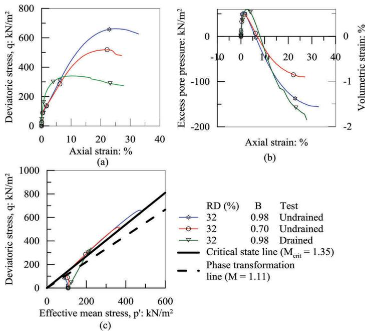
Figure 5. Effect of desaturation on: (a) stress strain behaviour; (b) excess pore pressure variation; (c) stress path in monotonic triaxial compression test.
