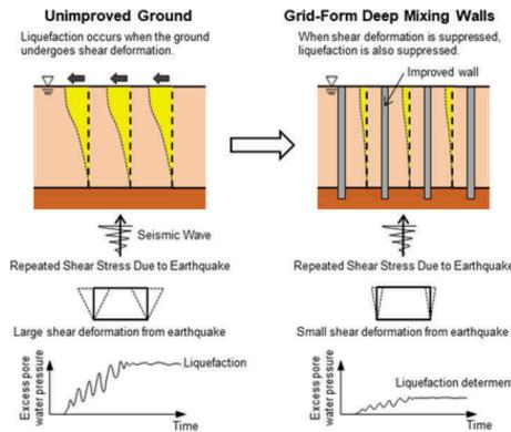
Figure 2. Liquefaction prevention mechanism by grid-form deep mixing walls.
