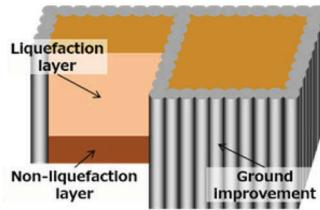
Figure 1. Structure of grid-form deep mixing walls.
