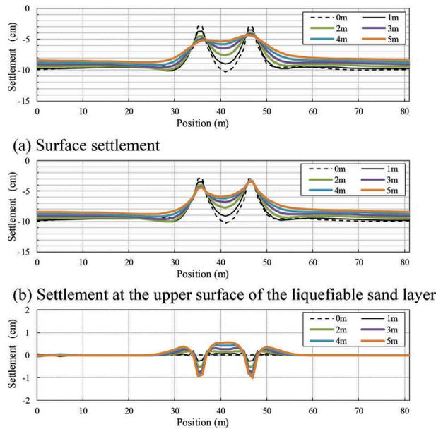
Figure 7. Distributions of settlement for the grid interval of 10 m in case L.
