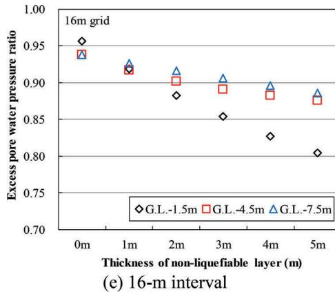
Figure 6. Relationship between excess pore water pressure ratio and thickness of the non-liquefiable sand layer.
