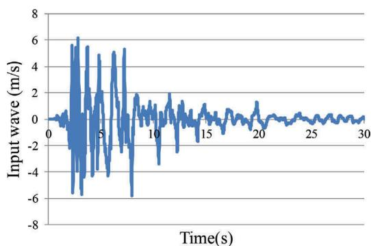
Figure 4. Input JR Takatori EW wave in the Hyogoken Nanbu earthquake (maximum acceleration is 6.155 m/s).
