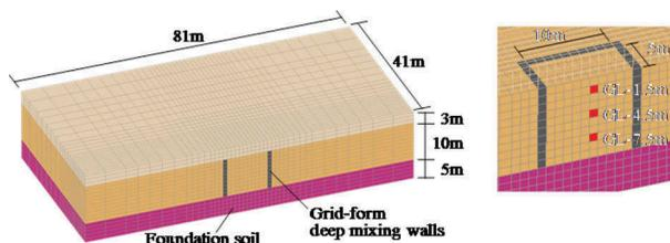
Figure 3. Numerical mesh (non-liquefiable sand layer: 3 m).
