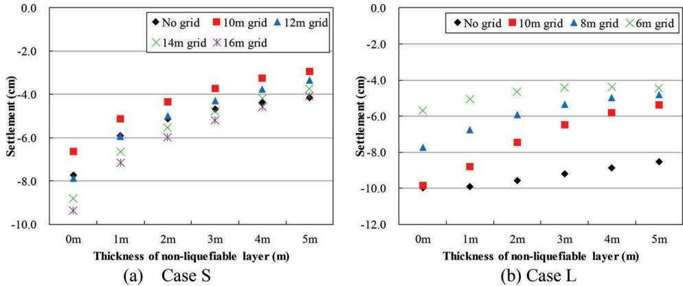
Figure 5. Relationship between the final settlement of the center of the grid-form deep mixing wall and thickness of the non-liquefiable sand layer.
