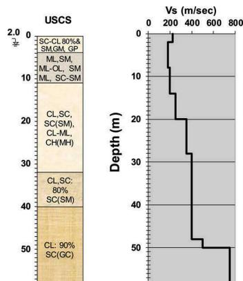
Figure 2. Schematic representation of the layered soil profile together with a general geotechnical characterization according to USCS classification as well as  $V_s$  profile.
