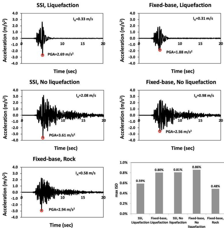
Figure 5. Acceleration time histories at the base of the structure and maxISD ratio for the different analysed configurations for Umbria Marche aftershock (ID 651) input motion at rock scaled to a PGA = 0.3g.
