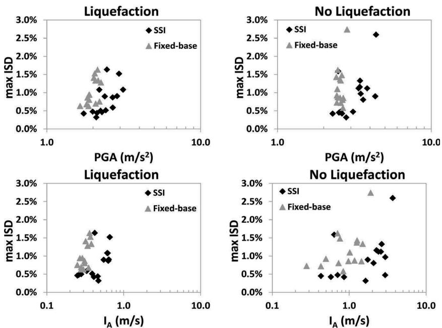
Figure 4. PGA - maxISD and  $I_A$  - maxISD pairs for the SSI and fixed-base models considering or not liquefaction.
