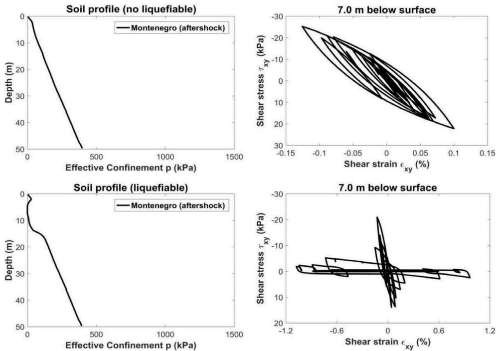
Figure 3. Variation of the effective confinement with depth and stress-strain hysteretic loops at 7.0m depth for the ID 229 input motion for the liquefiable (bottom) and the non-liquefiable (top) cases.
