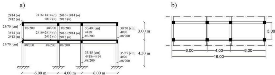
Figure 1. Schematic representation of the (a) cross-section with reinforcement details and (b) plan view of the reference MRF building used for the study (personal communication Kappos A and Panagopoulos G).
