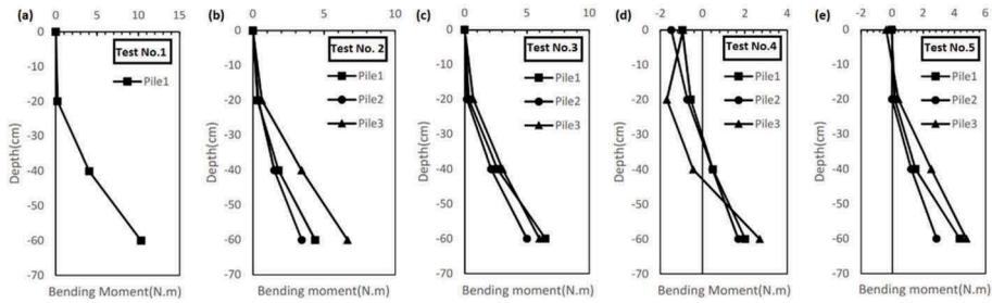
Figure 8. Profiles of the maximum bending moments in the model piles
