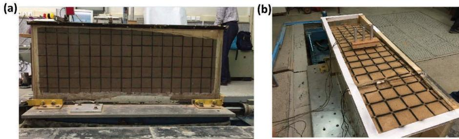
Figure 3. One of the physical models of the current study on the shake table: (a) front view (b) top view
