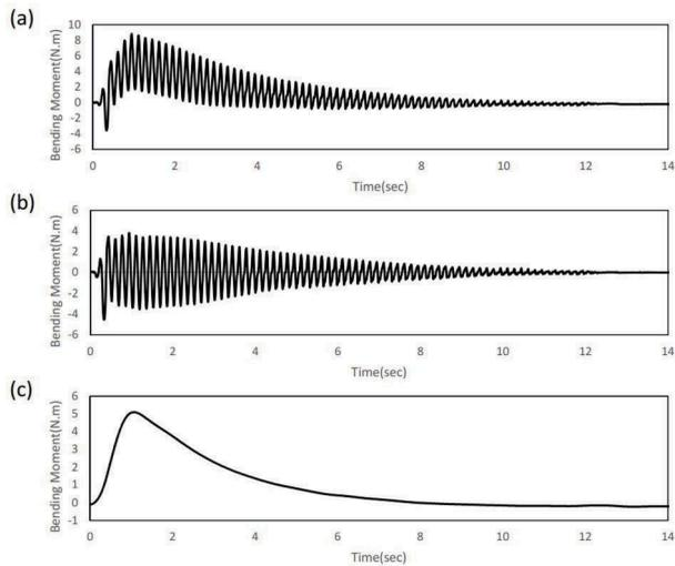
Figure 7. Time history of bending moment in pile 1 of Test no.3 at the base of liquefiable layer: (a) originally recorded (b) cyclic component (c) monotonic component.
