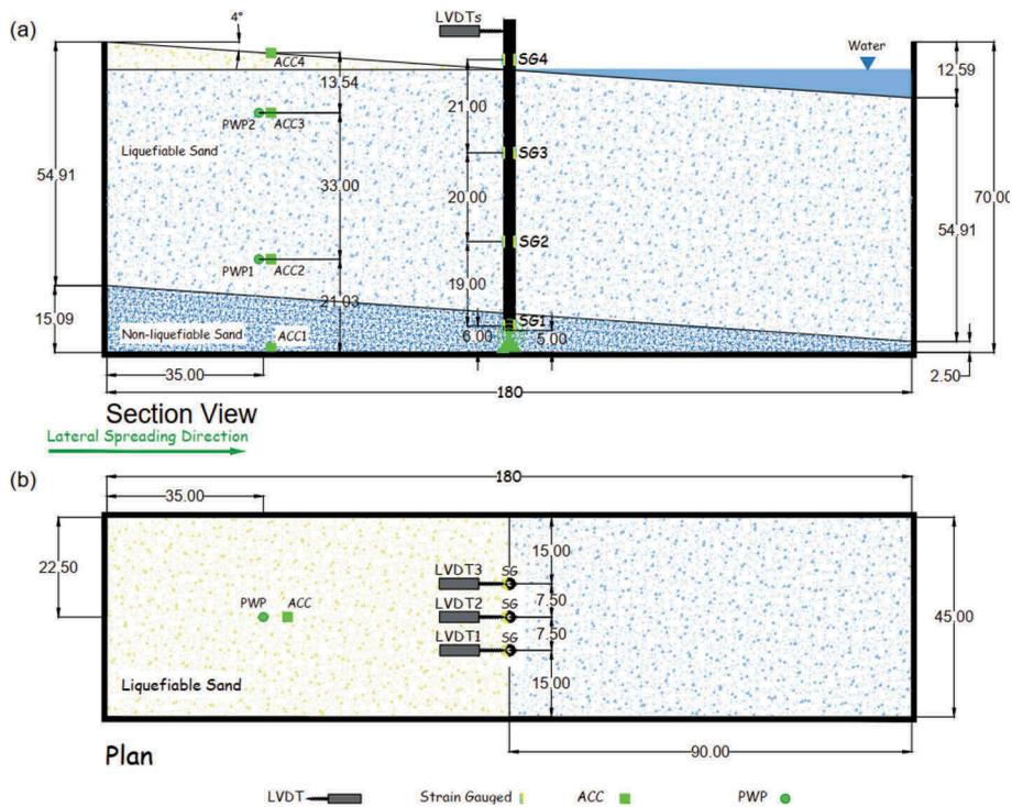
Figure 1. Plan and cross sectional views of a physical model test on a group of piles (without a cap) arranged perpendicular to the direction of lateral spreading
