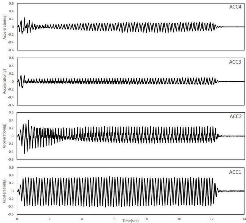
Figure 4. Typical time histories of acceleration of soil in free field for Test no.3
