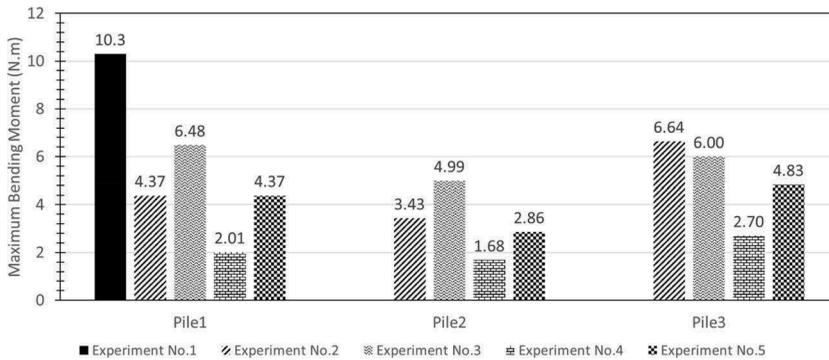
Figure 9. Maximum values of bending moments at the base of the model piles
