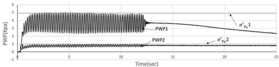
Figure 5. Typical time histories of excess pore water pressure in free field for Test no.3
