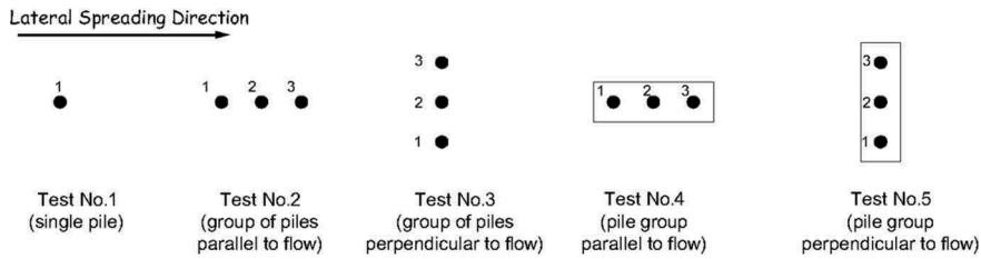
Figure 2. Schematic representation of configuration of piles in all experiments of the current study
