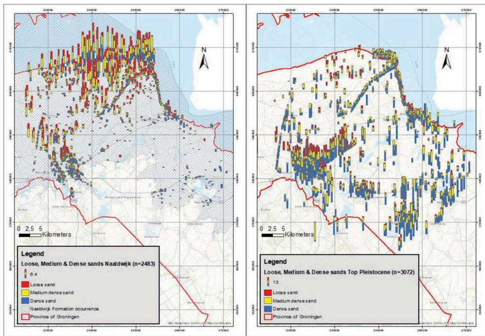
Figure 4. Stacked bars showing the total thicknesses of loose (red), medium dense (yellow) and dense (blue) sand in the Naaldwijk Formation (a) and Pleistocene sand (b). (Length of the bar indicates the total sand thickness in m).
