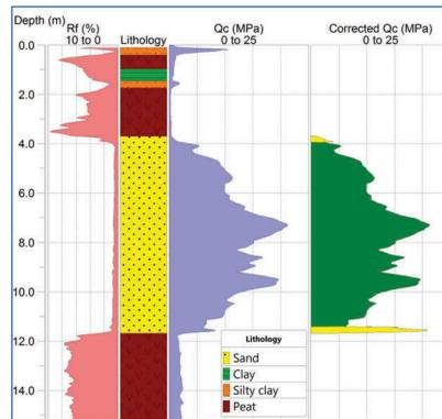
Figure 3. Example of original and corrected CPT for layered soil.
