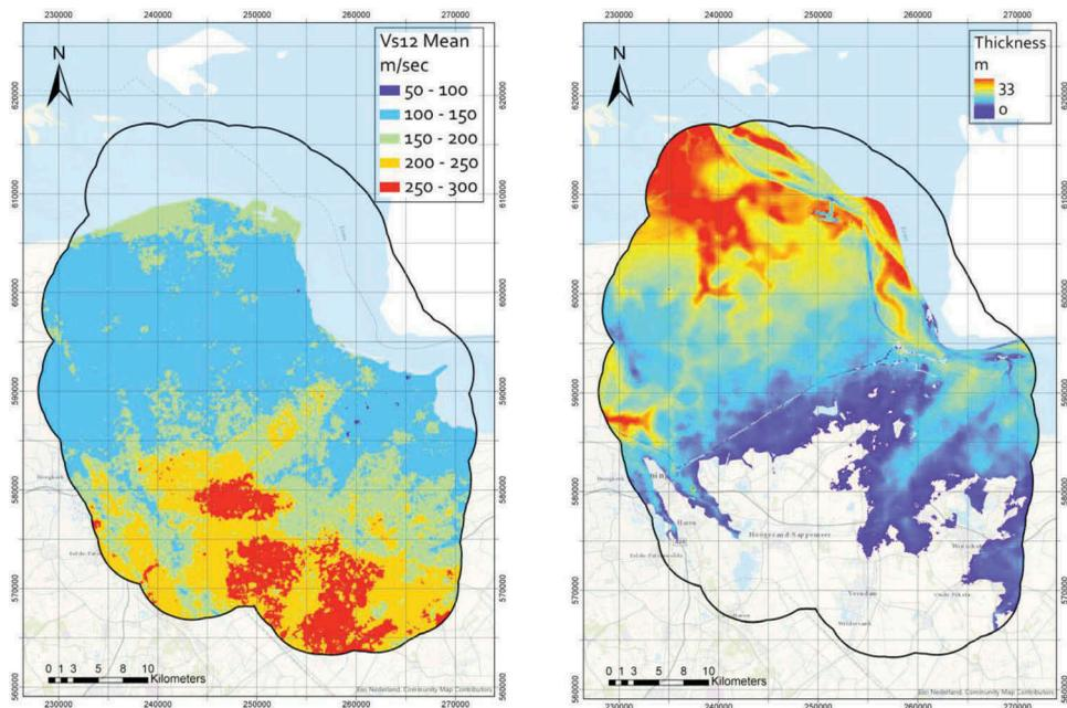
Figure 2.  $V_{s12}$  mean value (Kruiver, 2017a) (a) and thickness of the Holocene Naaldwijk Formation (Maljers et al., 2016) (b) in the geological model of the subsurface.
