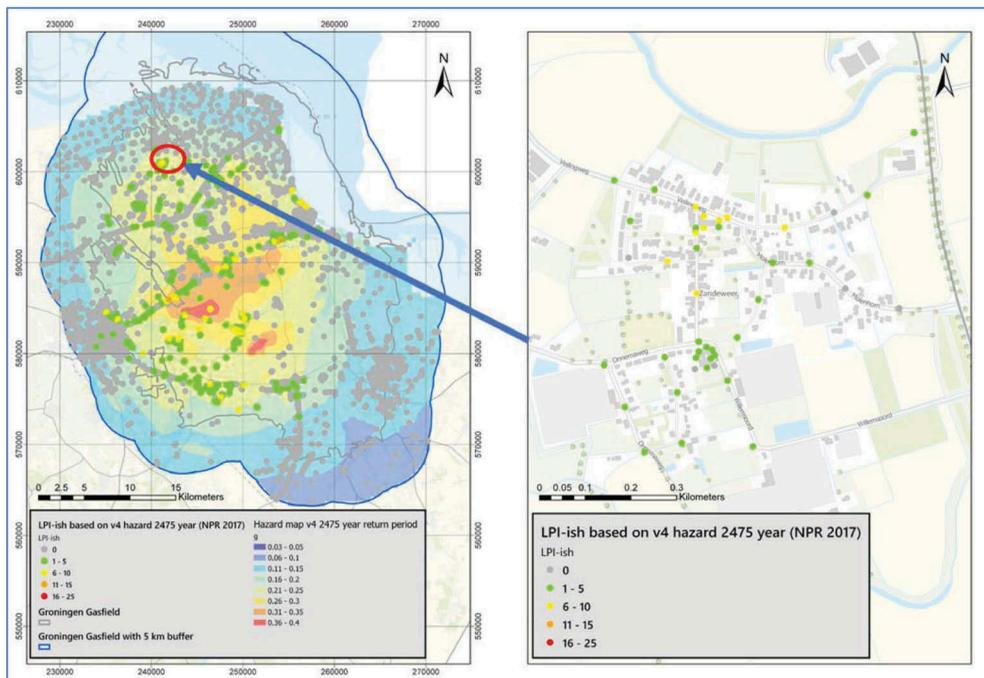
Figure 5. LPI<sub>ish</sub> map of Groningen based on the v4 hazard (NPR 2017) (left) with a detailed map of the town of Zandeweer in the northern part of Groningen as an example (right).
