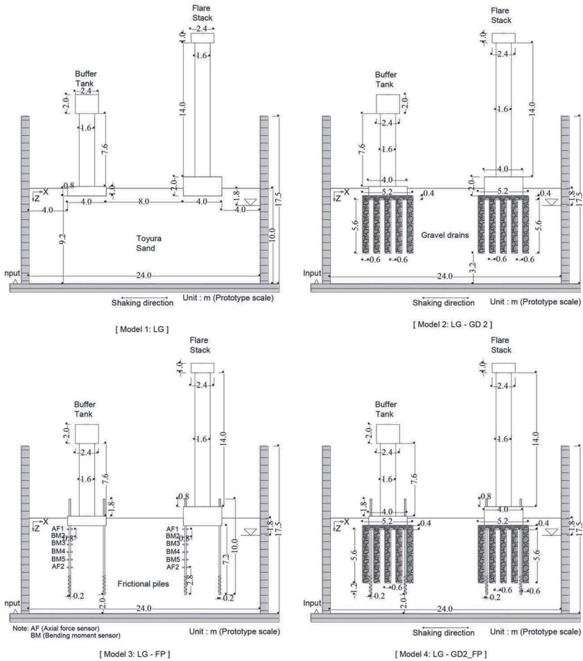
Figure 2. Centrifuge model configurations in prototype scale
