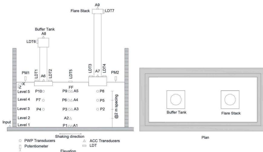
Figure 1. Typical centrifuge model layout
