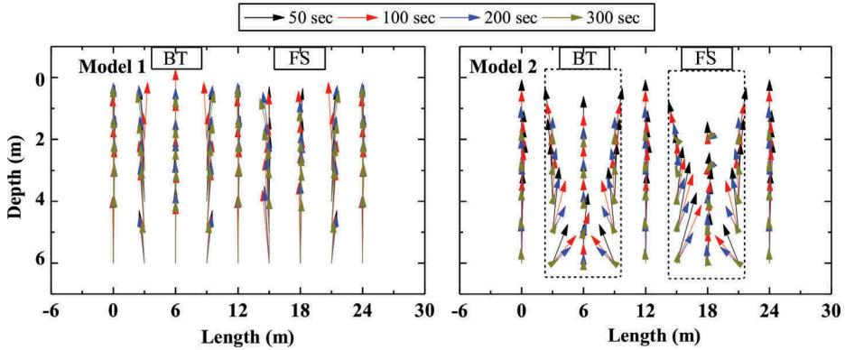
Figure 5. Pore fluid streamlines at different times for Models 1 and 2 during Tokachi-Oki ground motion
