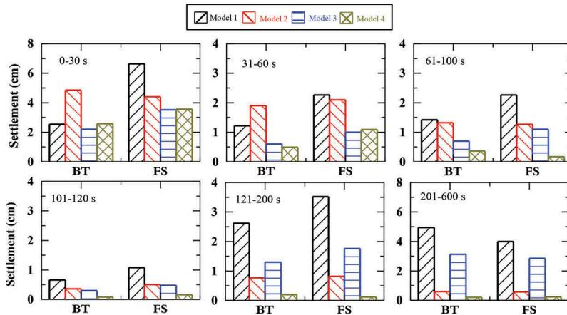
Figure 7. Average settlement of BT and FS footings for different time periods during Tokachi-Oki ground motion
