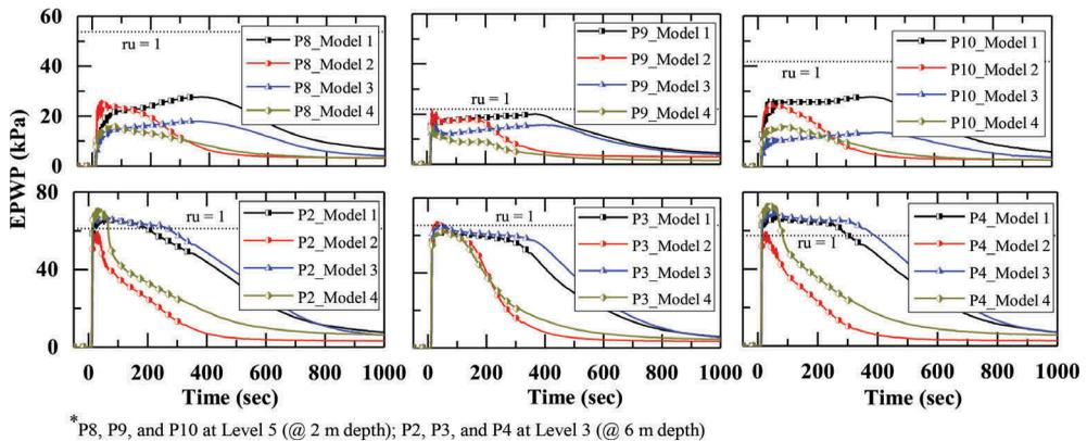
Figure 4. EPWP time histories of all the Models during Tokachi-Oki ground motion
