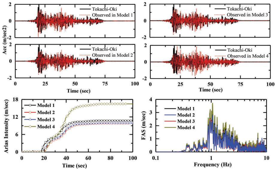
Figure 3. Acceleration time histories, Arias intensity and Fourier amplitude spectra (FAS) of input waves for all Models 1-4
