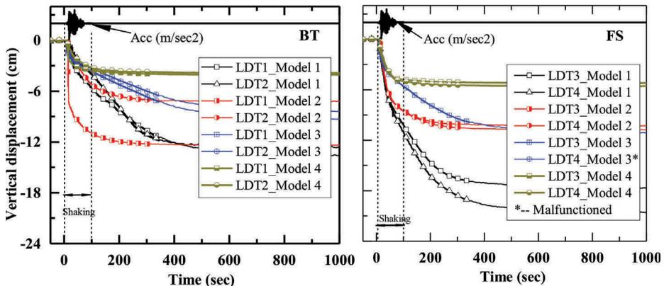
Figure 6. Settlement time histories of BT and FS footings during Tokachi-Oki ground motion
