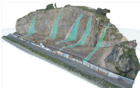
Figure 9. Rockfall trajectories, determined using industry standard 2D analysis, superimposed over the 3D site model.
