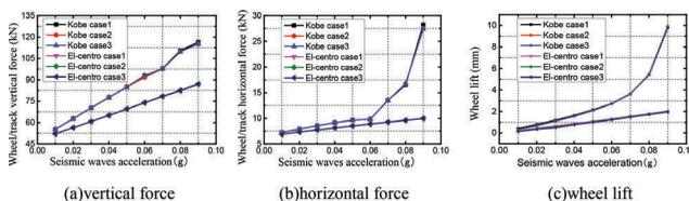
Figure 8. Dynamic reponse of wheel and track
