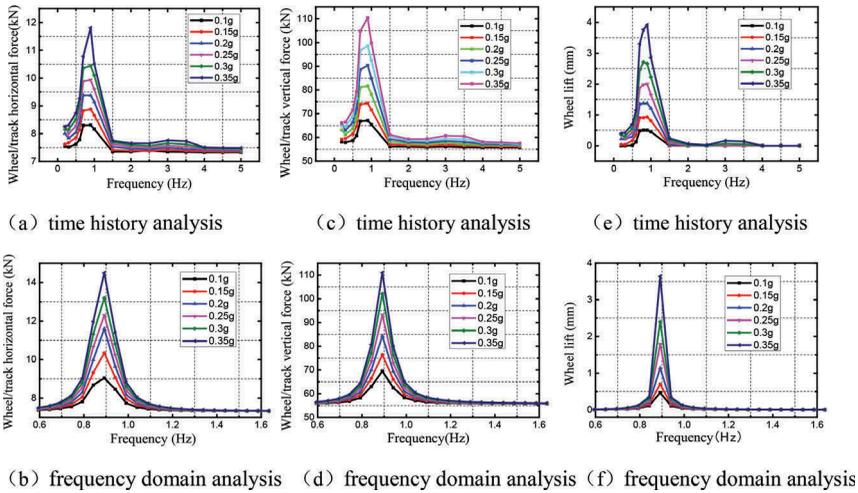
Figure 5. Frequency response of horizontal contact force vertical contact force and wheel lift
