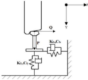
Figure 2. Schematic diagram of wheel and track contact
