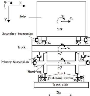
Figure 1. Vehicle-track dynamics model
