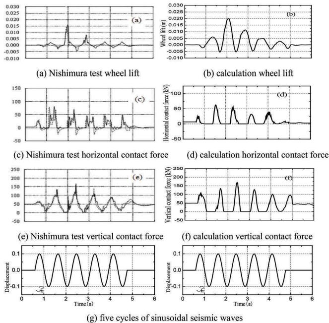
Figure 4. The time history of wheel motions (Nishimura's test and calculation, input:1.2Hz 100mm)
