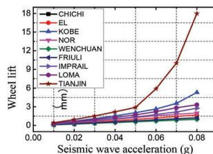
Figure 6. Wheel/track horizontal displacement      Figure 7. Wheel lift
