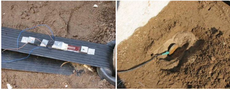
Figure 2. Pictures of the strain gages mounted on a geostrip (a) and of the soil pressure cells (b).
