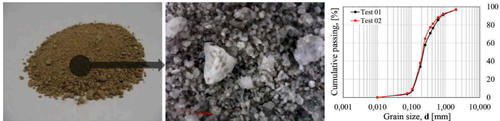
Figure 2. Photograph of Sofia sand and grain size distribution curve
