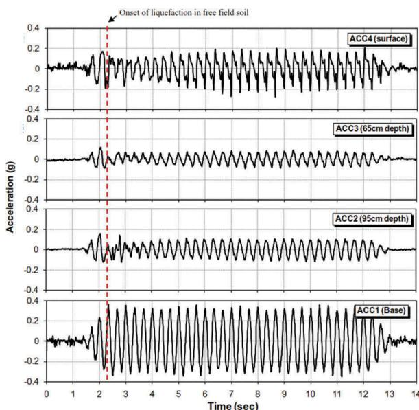
Figure 3. Time histories of acceleration in free field soil for model A
