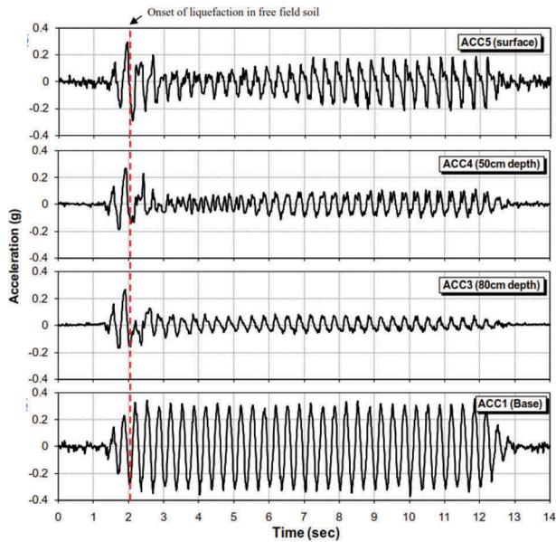
Figure 4. Time histories of acceleration in free field soil for model B
