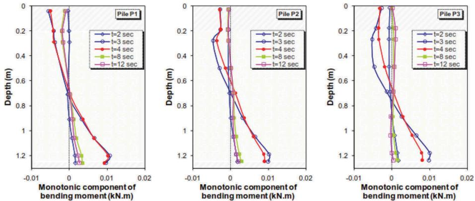
Figure 7. Profiles of bending moments along the piles in model A
