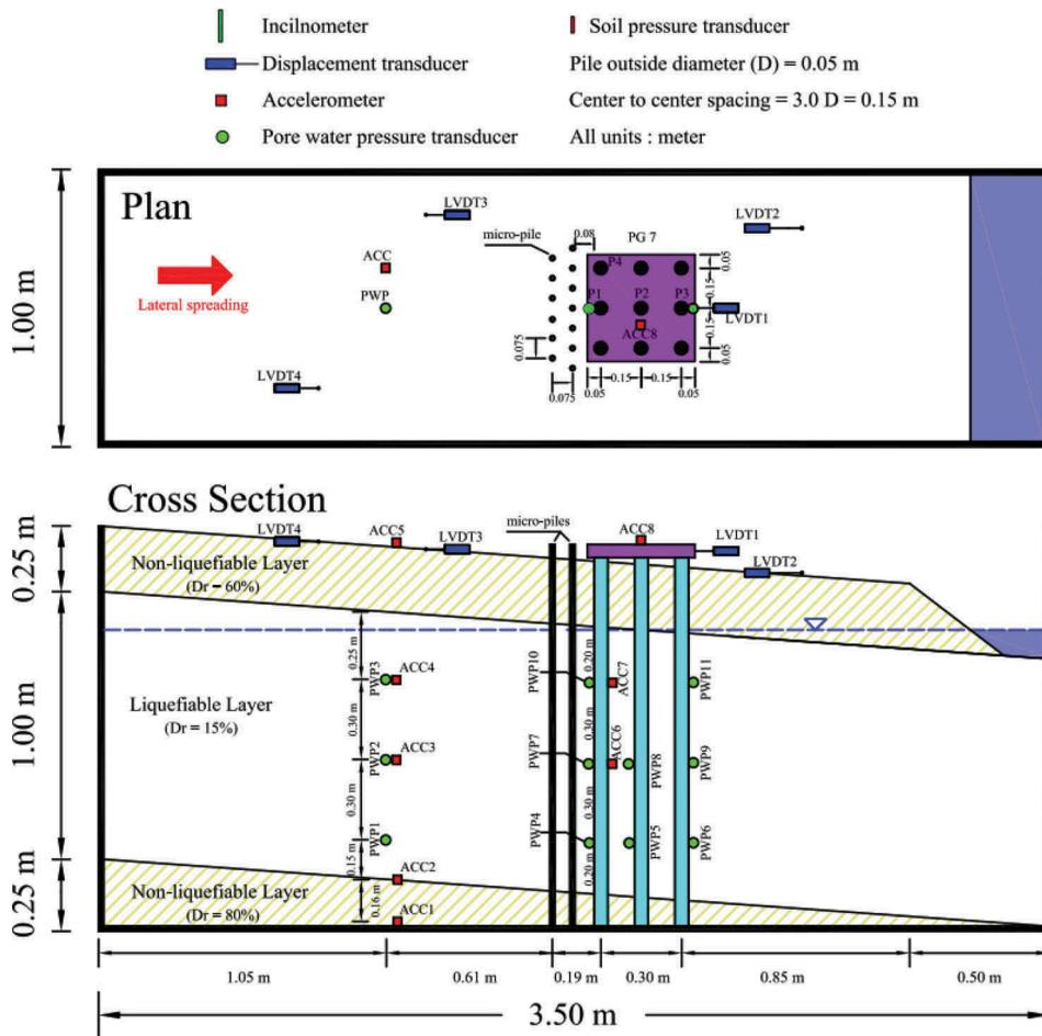
Figure 2. Plan view and cross section of model B and the instrumentation layout
