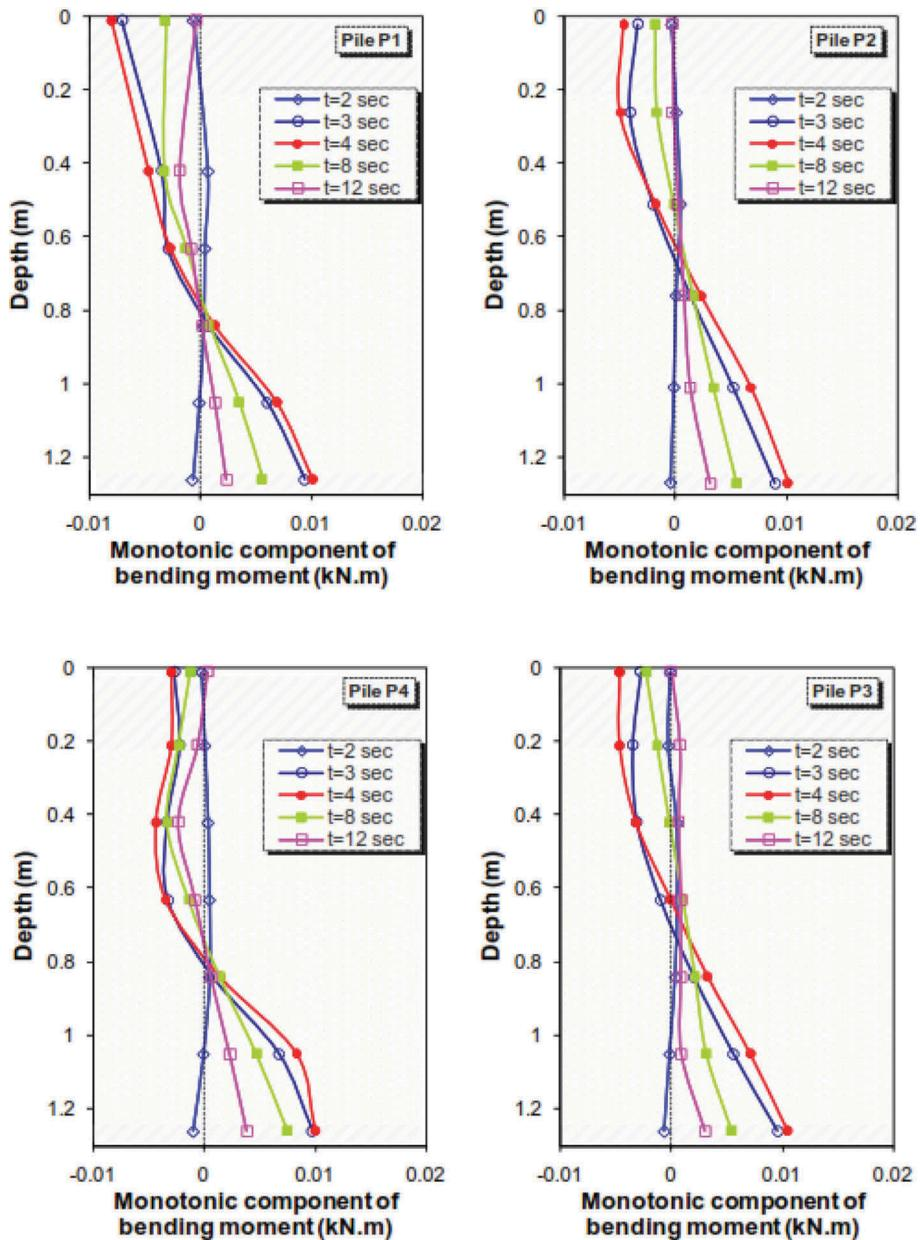
Figure 8. Profiles of bending moments along the piles in model B
