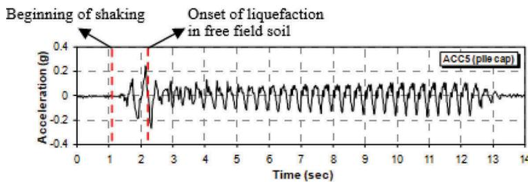
Figure 5. Time history of pile cap acceleration in model A
