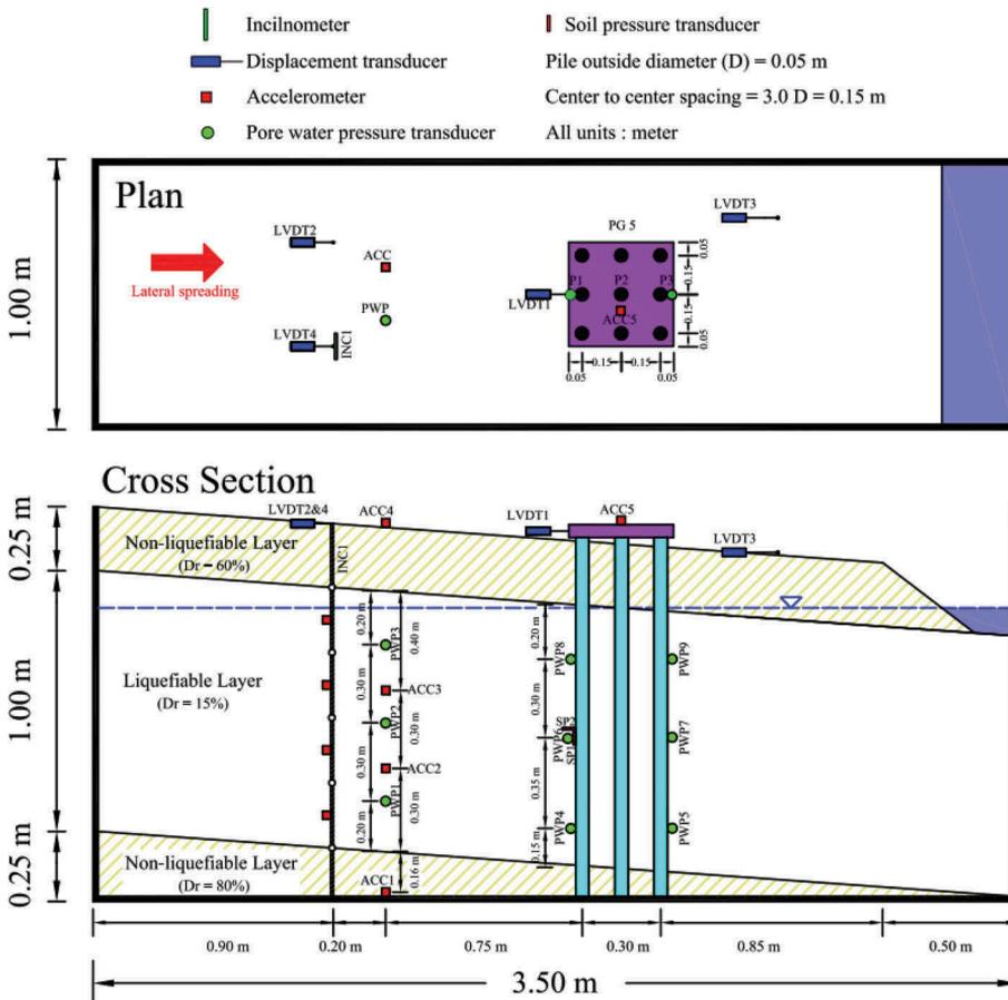
Figure 1. Plan view and cross section of model A and the instrumentation layout
