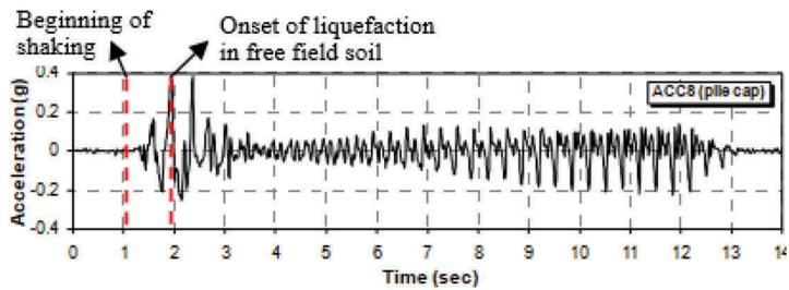
Figure 6. Time history of pile cap acceleration in model B
