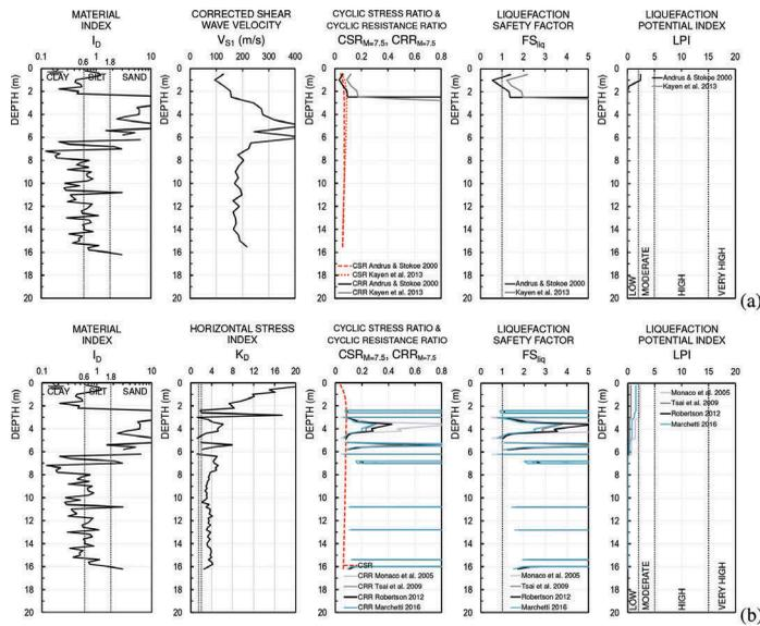
Figure 2. Vittorito – Results of the liquefaction analyses based on (a) the shear wave velocity  $V_s$ , and (b) the horizontal stress index  $K_D$ .
