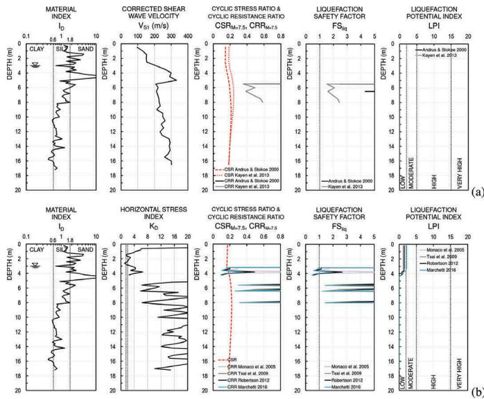
Figure 3. L'Aquila – Ponte Rasarolo – Results of the liquefaction analyses based on (a) the shear wave velocity  $V_s$ , and (b) the horizontal stress index  $K_D$ .
