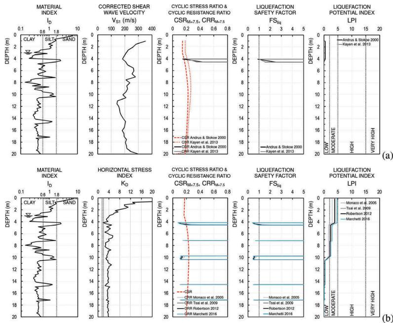
Figure 4. Fossa – Results of the liquefaction analyses based on (a) the shear wave velocity  $V_s$ , and (b) the horizontal stress index  $K_D$ .
