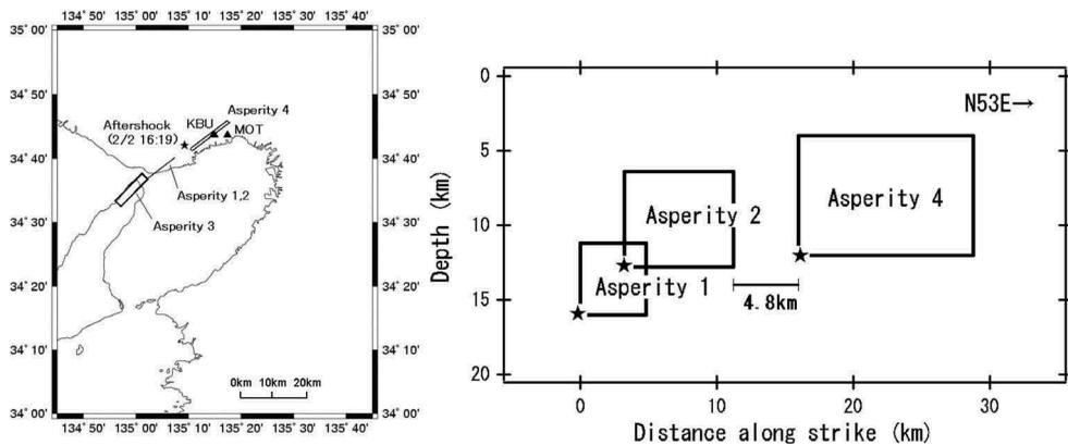
Figure 2. (left) The characterized source model by Yamada et al. (1999) for the 1995 Kobe earthquake, the epicenter of the aftershock used and the CEORKA strong motion sites KBU and MOT. (right) Its cross section for the Kobe side. The characterized source model has three asperities in the Kobe side. The stars indicate the rupture starting point for each asperity.
