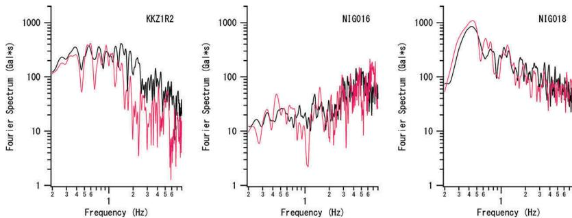
Figure 9. The recorded (black) and simulated (red) Fourier spectra at KKZ1R2, NIG016 and NIG018 for the 2007 Chuetsu-oki earthquake. The simulation was based on the characterized source model.
