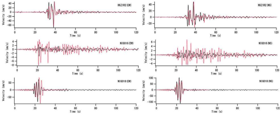
Figure 10. The recorded (black) and simulated (red) velocity waveforms (0.2-1Hz) at KKZ1R2, NIG016 and NIG018 for the 2007 Chuetsu-oki earthquake. The simulation was based on the pseudo point-source model.
