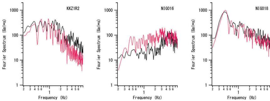
Figure 11. The recorded (black) and simulated (red) Fourier spectra at KKZ1R2, NIG016 and NIG018 for the 2007 Chuetsu-oki earthquake. The simulation was based on the pseudo point-source model.
