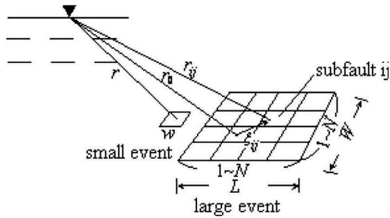
Figure 1. Superposition of Green's functions. The large rectangle shows an asperity.
