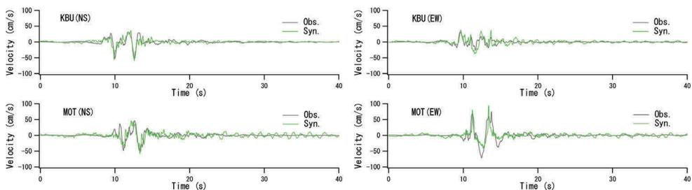
Figure 5. The recorded (black) and simulated (green) velocity waveforms at KBU and MOT for the 1995 Kobe earthquake. The simulation was based on the pseudo point-source model.
