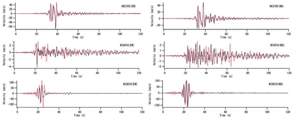
Figure 8. The recorded (black) and simulated (red) velocity waveforms (0.2-1Hz) at KKZ1R2, NIG016 and NIG018 for the 2007 Chuetsu-oki earthquake. The simulation was based on the characterized source model.
