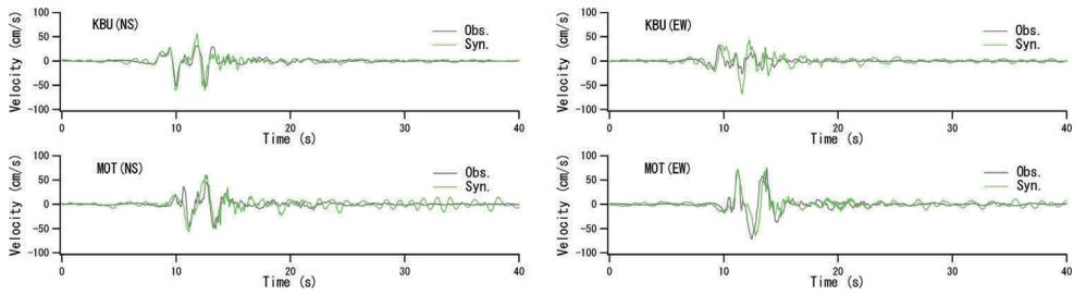
Figure 3. The recorded (black) and simulated (green) velocity waveforms at KBU and MOT for the 1995 Kobe earthquake. The simulation was based on the characterized source model.
