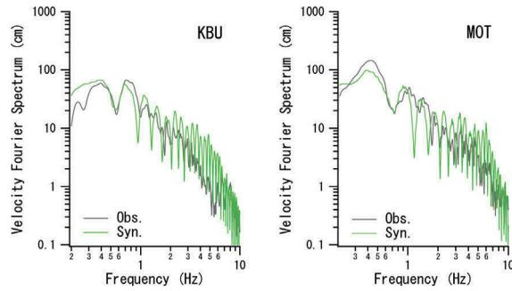
Figure 6. The recorded (black) and simulated (green) velocity Fourier spectra at KBU and MOT for the 1995 Kobe earthquake. The simulation was based on the pseudo point-source model.
