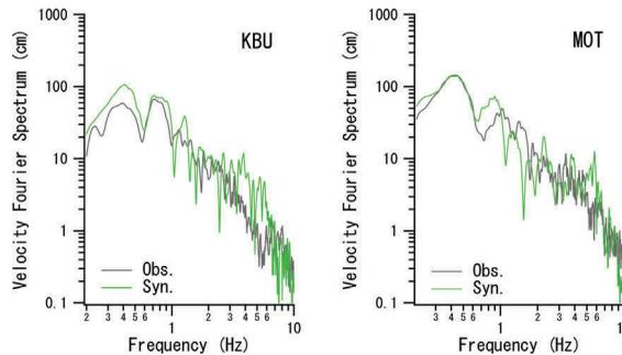
Figure 4. The recorded (black) and simulated (green) velocity Fourier spectra at KBU and MOT for the 1995 Kobe earthquake. The simulation was based on the characterized source model.
