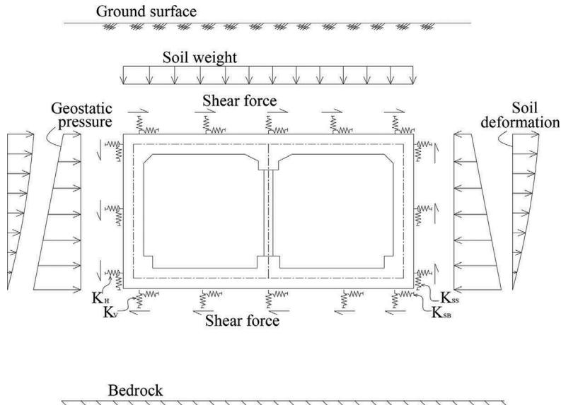
Figure 4. Boundary condition and applied loads to the tunnel
