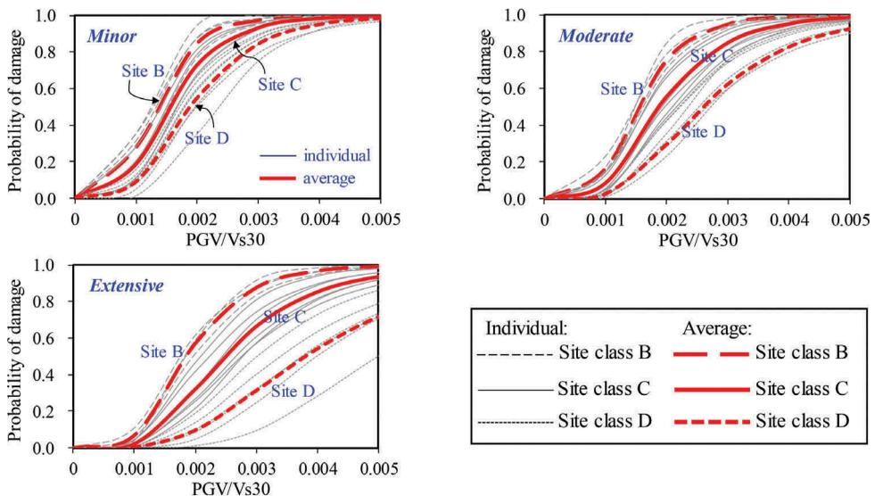
Figure 7. Fragility curves of the double box tunnel using  $PGV/V_{s30}$
