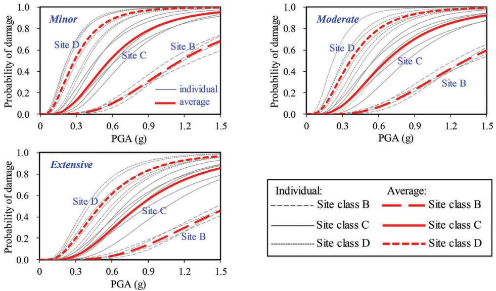
Figure 6. Fragility curves of the double box tunnel using PGA
