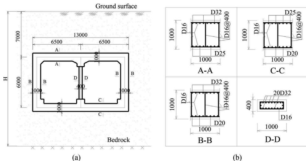
Figure 1. Tunnel cross section (a) and reinforcement detail of tunnel lining (b)
