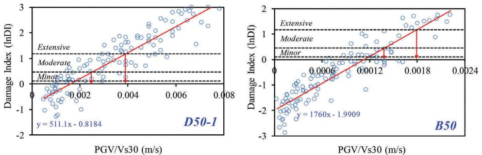
Figure 5. DI and seismic intensity measure and estimation of mean values for damage states
