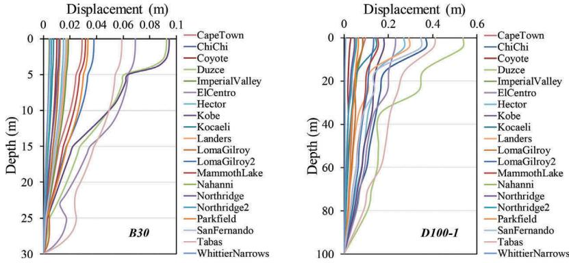
Figure 3. Peak displacement of site profiles
