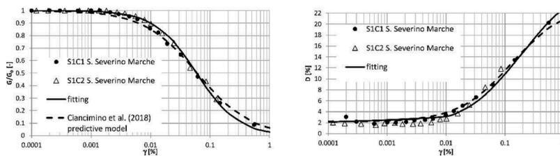
Figure 3. Normalized shear modulus (a) and damping ratio (b) versus shear strain.
