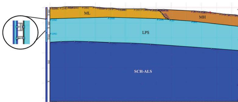
Figure 4. Free-field conditions at the lateral boundaries (normal and tangential viscous dampers).
