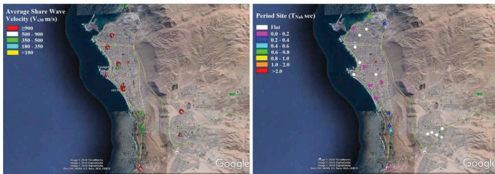
Figure 2. The  $V_{s30}$  hazard map for Iquique-Alto Hospicio is shown on the left and the  $T_N$  hazard map on the right.
