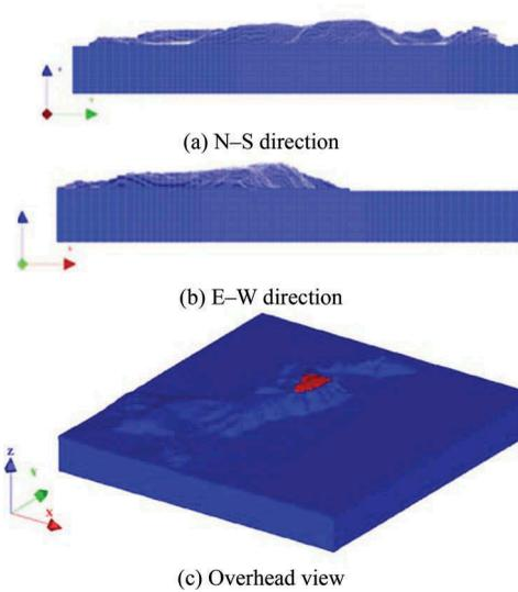
Figure 6. Analytical model. The red areas denote sediment layers
