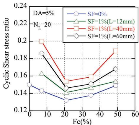
Figure 9. Relationship between Liquefaction strength and fine fraction content  $F_c$ .
