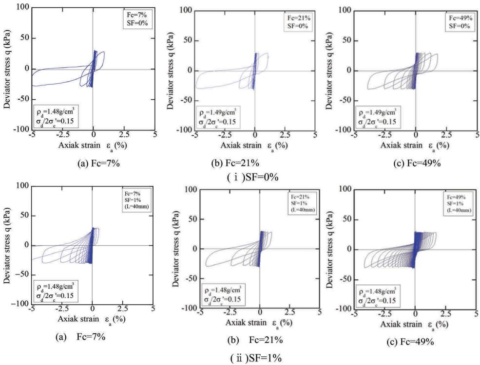
Figure 5. Relationship between axial strain and deviator stress.
