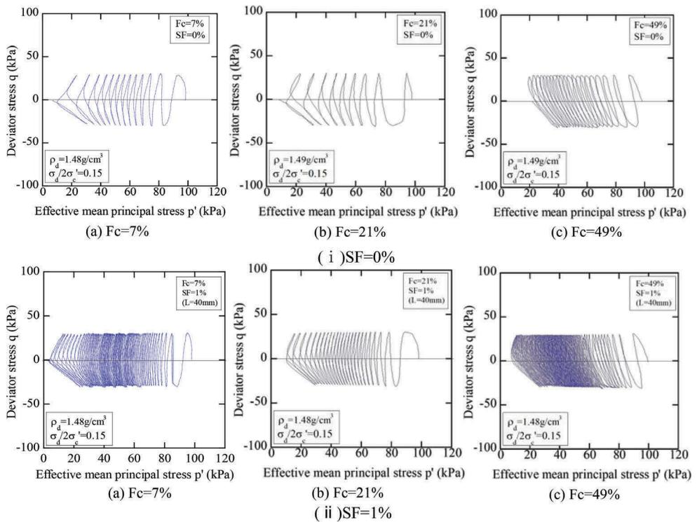
Figure 4. Effective stress paths on undrained cyclic shear behavior (SF=0%, SF=1%).
