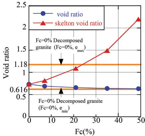
Figure 3. Relationship between void ratio and fine fraction content, Fc (%).
