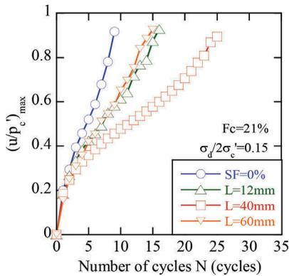
Figure 6. The relationships between number of cycles and maximum pore pressure ratio.
