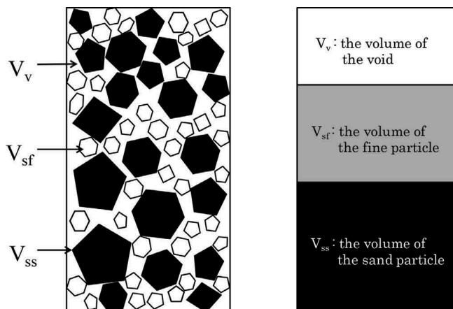
Figure 2. Skeleton model of soil.
