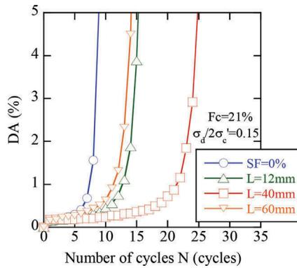
Figure 7. The relationships between number of cycles and double amplitude axial strain.
