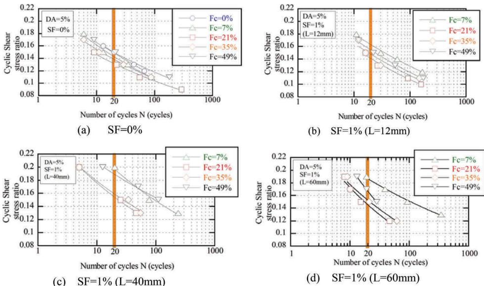
Figure 8. Liquefaction strength curve.
