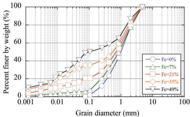
Figure 1. Particle size distribution of soil samples.
