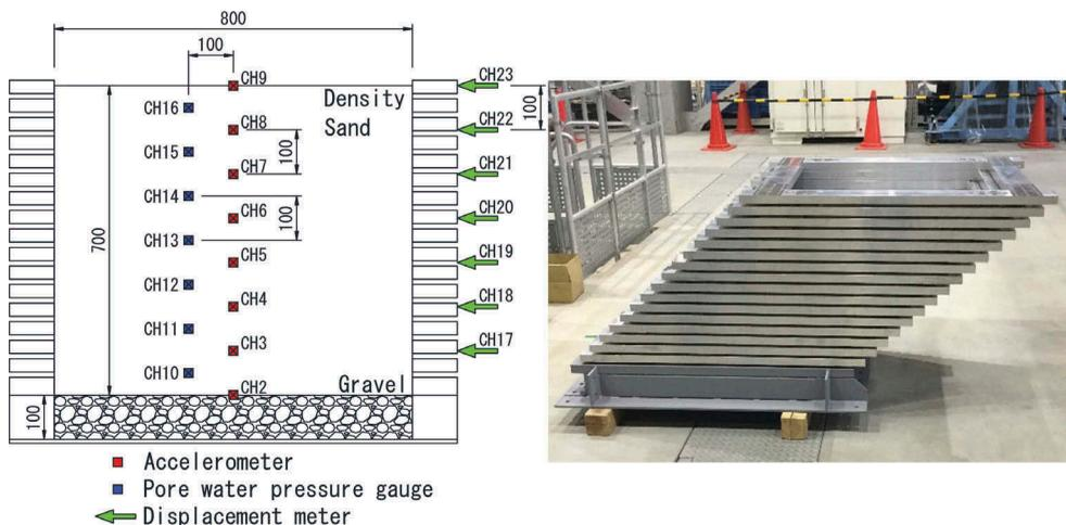
Figure 2. An experimental model of shaking table tests.
