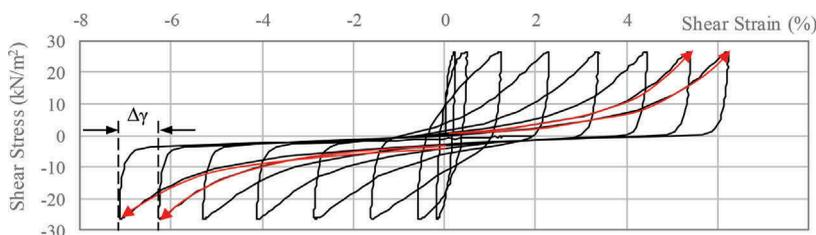
Figure 4. Relationship between shear stress and shear strain at cyclic undrained triaxial test
