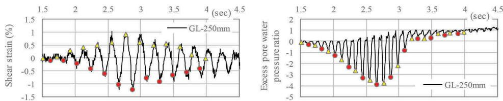
Figure 6. Time history of shear strain and excess pore water pressure ratio at Case 1 (The section of  $t = 1.5$  to 4.5 sec of Figure 6 is enlarged.)
