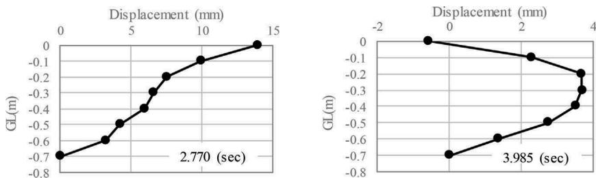
Figure 7. Depth distribution of horizontal displacement at shear box
