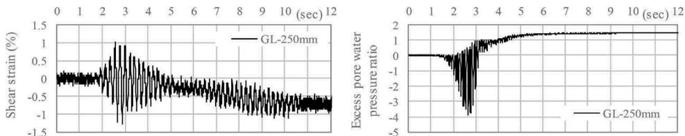
Figure 5. Time history of shear strain and excess pore water pressure ratio at Case 1
