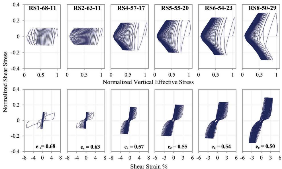
Figure 2. Stress-strain and stress-path responses of reconstituted specimens during repeated cyclic shear loading stages in constant-volume cyclic DSS tests
