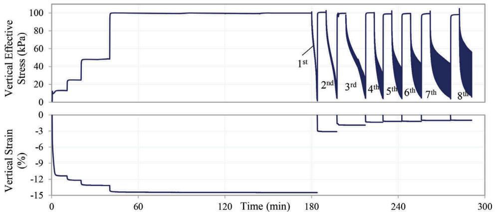
Figure 1. Vertical effective stress and vertical strain during 8 stages of repeated cyclic direct simple shear loading and reconsolidation for reconstituted silt
