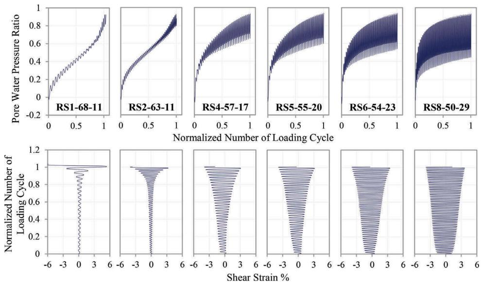
Figure 4. Accumulation of strain and generation of reconstituted specimens during repeated cyclic shear loading stages in constant-volume cyclic DSS tests
