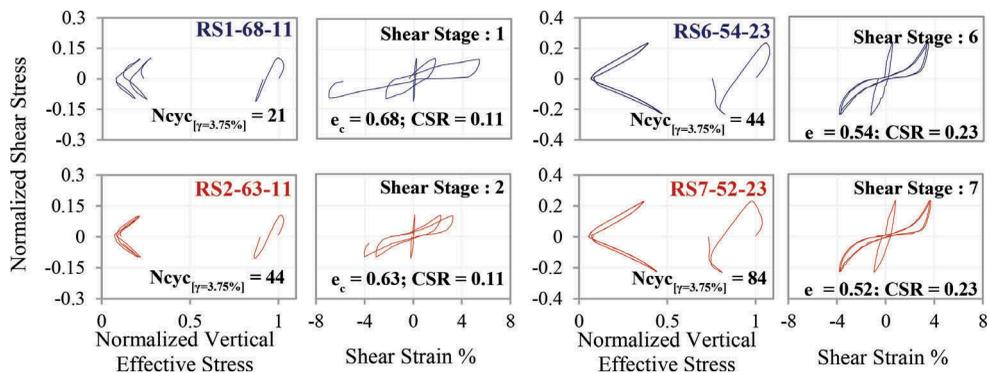
Figure 3. Stress-strain and stress-path responses of the first and the last two loading cycles for shearing stages 1-2 and 6-7 during repeated cyclic shear loading stages in constant-volume cyclic DSS tests
